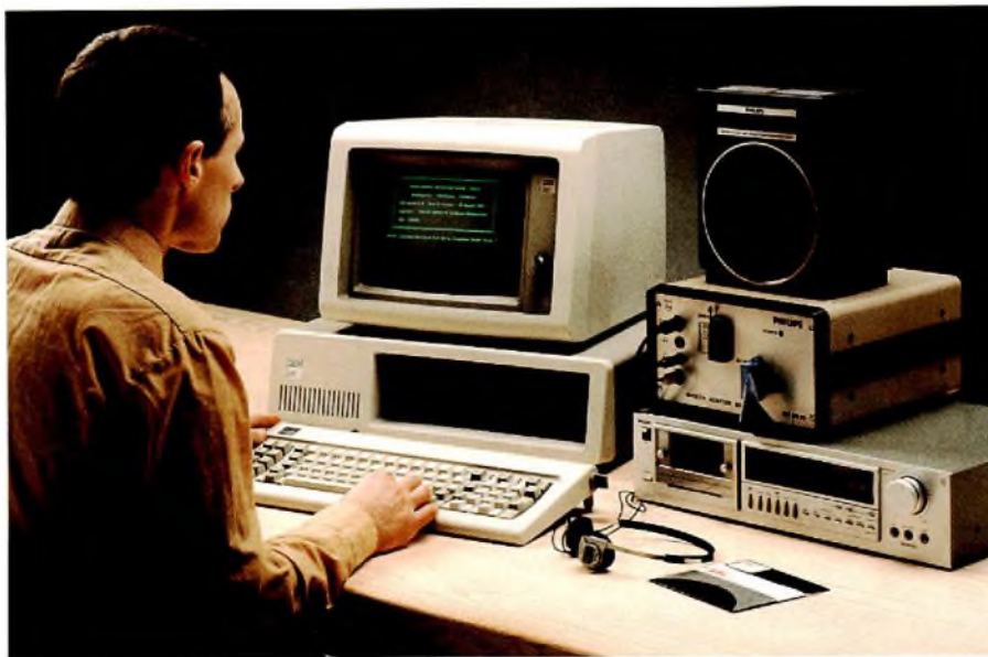
Fig.1 Our speech-development system comprises a hardware I/O for an IBM PC (shown here) or an HP 9816S computer and all the software (on floppy disk) for analyzing, coding and editing speech. A feature of this system is the graphic display of the speech parameters representing the synthesized speech
