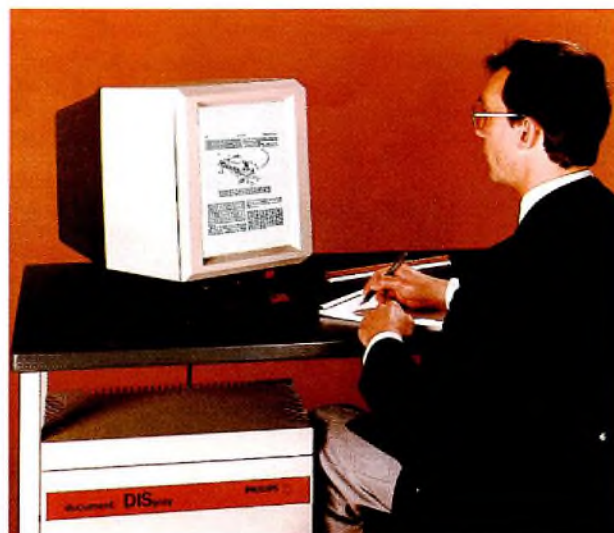
Pages called up on the Megadoc screen are displayed full size, black on white. A refresher memory in the cabinet beneath the desk-top keeps them on display for as long as the user requires
