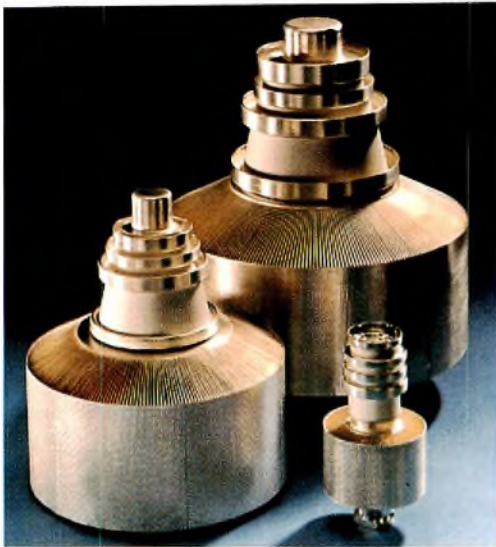
Fig.5 Forced-air-cooled anodes have copper fins brazed to their outsides. They can dissipate powers up to about 500 \text{ W/cm}^2
