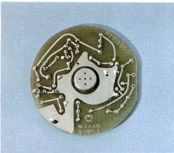
Fig.15 Assembled discrete amplifier and electret capsule: (a) front view; (b) rear view
