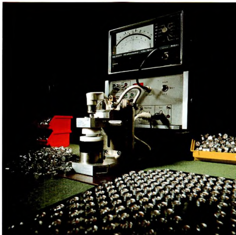
Fig.12 Quality control test of sensitivity and FET performance
