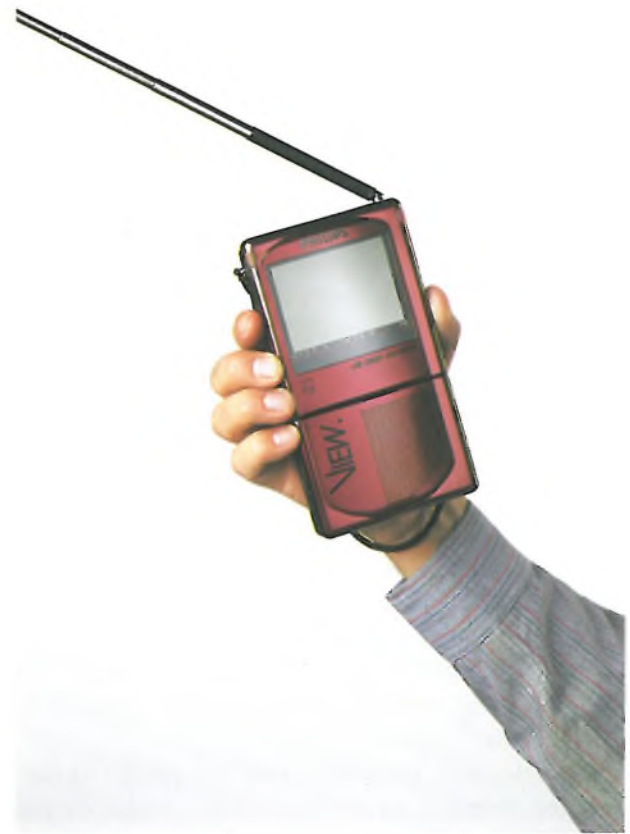
Fig. 7. The use of liquid-crystal displays (LCDs) opens new possibilities for television. The colour television receiver shown here has a screen with a diagonal of 7.5 cm (3 in) and requires only a few watts of power.
