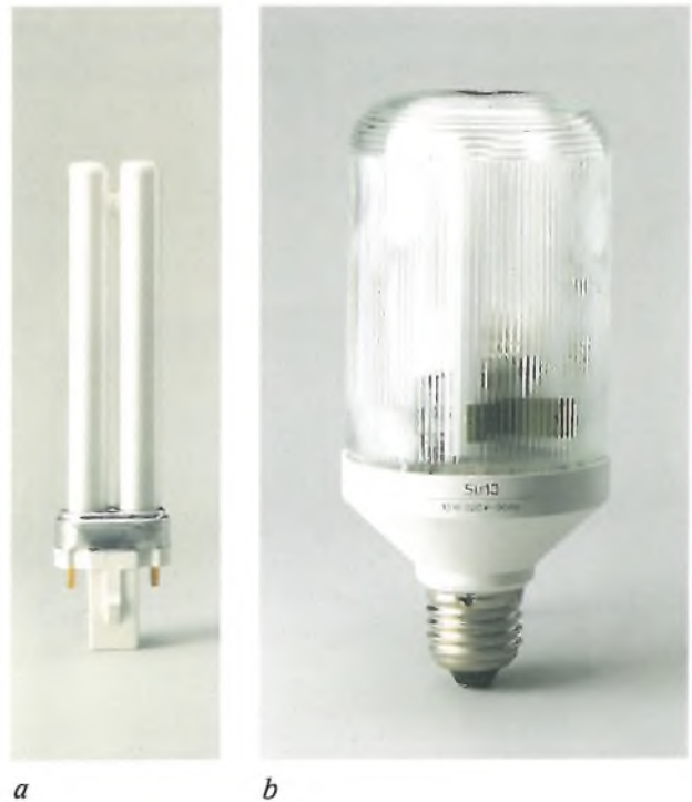
Fig. 3. In recent years developments in fluorescent lamps have led to compact lamps with more than four times the efficacy and five times the life of comparable incandescent lamps. Examples are the PL* lamp (a) and the SL* lamp (b). The SL* lamp has a built-in ballast and the same base as conventional incandescent lamps, so that existing fittings can be used.
