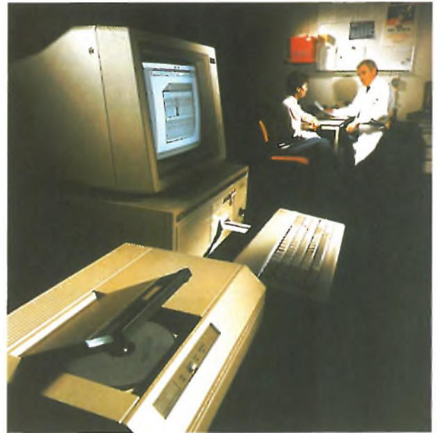
Fig. 12. Two highly promising versions of the Compact Disc are the CD-ROM and the CD-I, which each contain some 600 megabytes of information on a disc with a cross-section of about 12 cm. This photograph gives an impression of the use of a CD-ROM. For both CD-I and CD-ROM screens have an important part to play in displaying the information.
