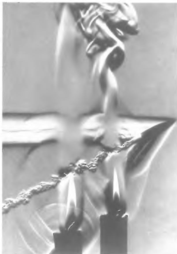
Fig. 1. This picture, made by the Schlieren method, shows a bullet travelling through the air above two candle flames. This photograph is taken from the book of note [2] (page 560).
