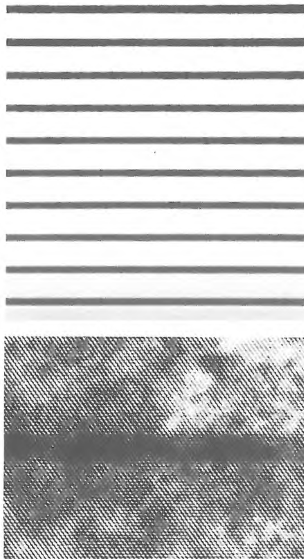
Fig. 8. Above: (110) cross-sectional TEM micrograph of a multiple quantum-well structure. The GaAs wells (dark) are 5.5 nm thick, the \text{Al}_x\text{Ga}_{1-x}\text{As} barriers (light) 17.5 nm. The micrograph was taken under dark-field conditions using the (002) diffraction. Below: high resolution (110) cross-sectional TEM micrograph (dark-field image) of a 2.7-nm quantum well of GaAs (dark) between two \text{Al}_x\text{Ga}_{1-x}\text{As} barriers (light). The samples were grown by K. Woodbridge and the micrographs were taken by J. P. Gowers and D. J. Smith (University of Cambridge).
