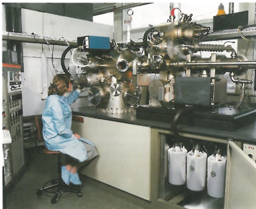
Fig. 3. General view of the MBE equipment (Varian GEN II) at the Philips Research Laboratories in Redhill. The growth occurs in the vacuum chamber on the left by effusing molecular beams from the tubular Knudsen cells. The growth rates for GaAs and \text{Al}_x\text{Ga}_{1-x}\text{As} can be deduced from RHEED intensity variations measured in the growth chamber. The vacuum system on the right is used for the introduction and preparation of substrates.
