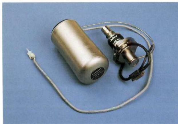
Fig. 6. The USFA cryogenerator integrated with an infrared detector in a vacuum vessel (Dewar) on the right. The complete Dewar with detector has the Mullard type number R170.
