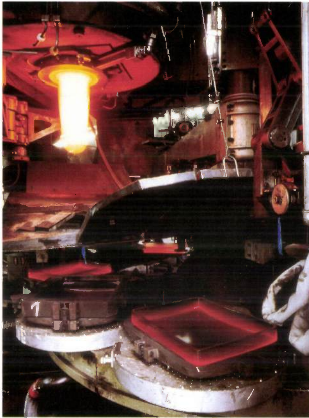
Fig. 5. Screens for colour picture tubes being pressed in the television pressed-glass works at Aachen, West Germany.
