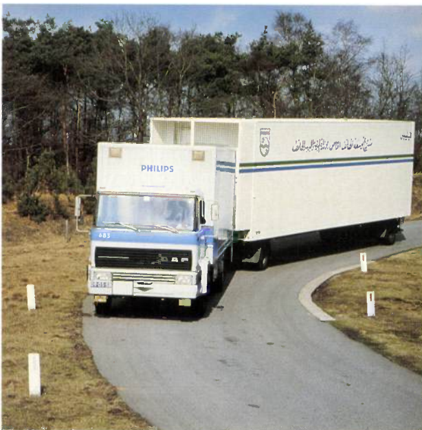
Fig. 15. Because automatic telephone exchanges have become much smaller, it is possible to use ready-made mobile 'container' exchanges for certain applications. This container is being shipped from the Netherlands to Saudi Arabia.
