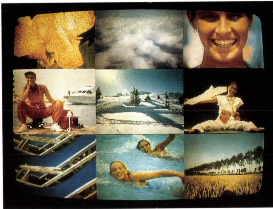
Fig. 23. The use of field memories also makes it possible to combine parts of pictures. The example given here is 'multi-picture-in-picture', where the signals originating from several different transmitters are displayed simultaneously. This can be a very useful facility when making a selection from a large number of programmes.
