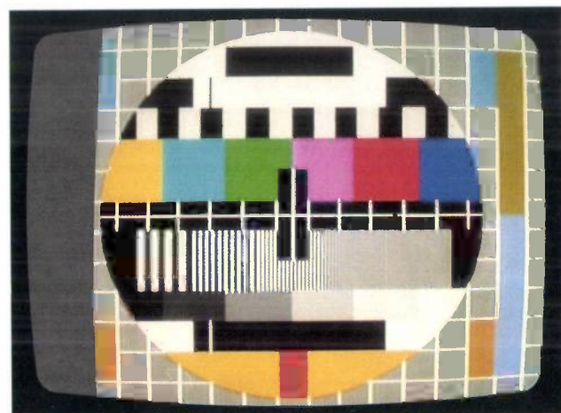
Fig. 18. a ) The original colour pictures of fig. 17 a after bandwidth limitation of the composite signal to 3 MHz. b ) Result after a CAROT operation on the original pictures, followed by bandwidth limitation of the new composite signal to 3 MHz and an inverse CAROT operation.
