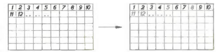
Fig. 1. Principle of television. The surface of the picture to be televised is resolved into a number of small elements which are numbered in succession. The brightness of each individual element is telegraphed. At the receiver where the picture surface is subdivided into similar elements each element is given the brightness transmitted for its respective number, so that the received picture exactly reproduces the original.
