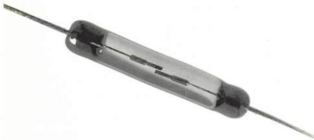
Fig. 14. Mini-reed contact from a Philips reed relay. The magnetic 'reeds' can clearly be seen in the hermetically sealed glass encapsulation. To operate the contact, a coil is required, to produce a magnetic field; one coil is often used to operate more than one contact simultaneously.
