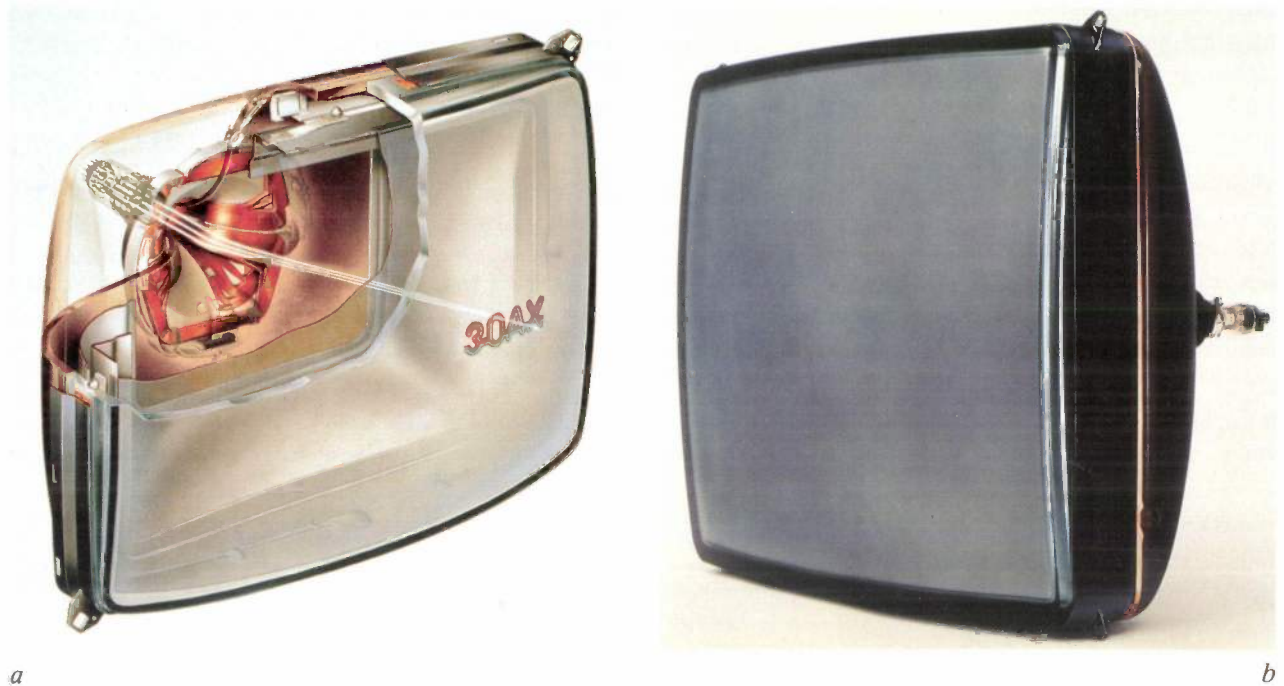
Fig. 13. a ) In a shadow-mask tube a colour television image is generated by the combined action of three electron beams, a mask with a very large number of tiny holes and a picture tube coated on the inside with accurately positioned red, green and blue phosphor dots. The electron beams scan the entire screen 25 or 30 times a second under the control of a number of deflection coils on the neck of the tube. b ) There is continuing refinement and improvement of the shadow-mask tube: the aim is to make the screen as flat and rectangular as possible with the minimum overall tube length. The type 45AX 'flat square tube' shown here also has an extremely thin neck (29.1 mm); this means that less energy is required for the deflection of the electron beam.
