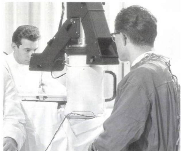
Fig. 6. The Alfax, an X-ray image intensifier with a diameter of 9 inches, equipped with double mirror optics and a cine camera. During fluoroscopy two observers (e.g. radiologist and surgeon) could examine the image at the same time and film it when required.
