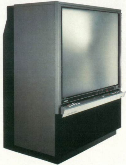
Fig. 16. Modern projection-television set. It contains three separate 7-inch high-resolution cathode-ray tubes, which each reproduce a sub-picture in one of the basic colours red, green and blue. The three sub-pictures are projected on the screen under electronic control to give exact registration. The actual screen is rectangular and flat with a diagonal of 37 inches (about 94 cm). Below the screen there is a drawer (shown open) containing various controls for vision and sound. The set can also be operated with remote control.
