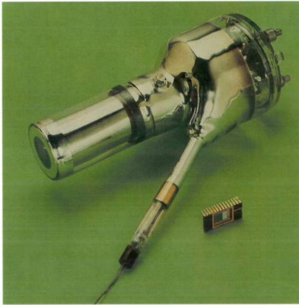
Fig. 20. A comparison of an image iconoscope with a modern semiconductor image sensor gives a good impression of the dramatic reduction in size in 50 years of television-camera technology.
