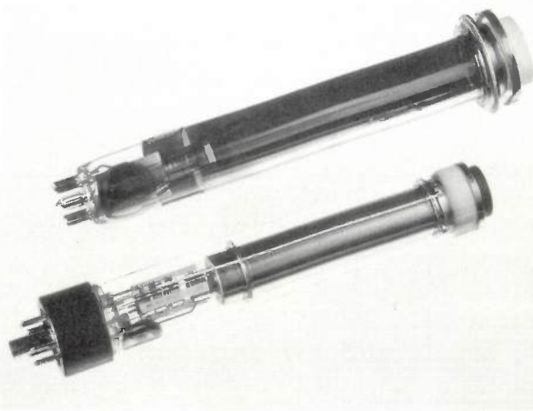
Fig. 11. 1-inch and 2-inch Plumbicon tubes. The Plumbicon tube replaced the vidicon and solved the problem of excessive inertia. Enlargement of the photosensitive area enabled the number of lines in the frame to be doubled, thus greatly increasing the picture definition. This was turned to great advantage in digital imaging techniques.
