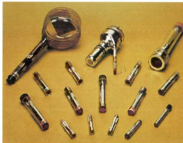
Fig. 3. While the dimensions of television camera tubes diminished, the characteristics improved. Here in the top row we have, from left to right, an iconoscope, an image iconoscope and an image orthicon. Below there is a great variety of camera tubes: first a row of four vidicons, then a row of five Plumbicon tubes and finally another row of four vidicons.
