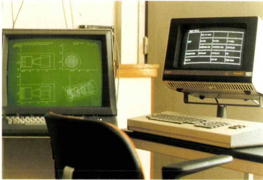
Fig. 2. The GELOP terminal. Left, the graphic display, right, the alphanumeric screen. 'Menus' displayed on the alphanumeric screen enable the user to make his wishes known to the computer system. The results of the calculations are displayed on the graphic display.
