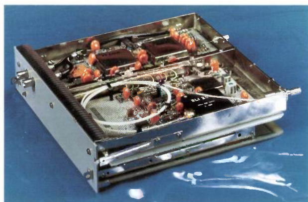
Fig. 7. Receiving equipment for a 565-Mbit/s optical-transmission system.
