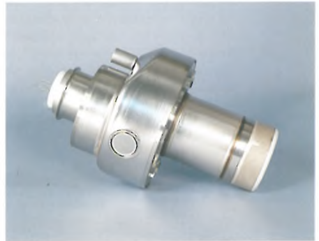
Fig. 1. The new Philips MRC200 diagnostic X-ray tube with an anode mounted in spiral-groove bearings lubricated by liquid metal. The anode diameter is 200 mm. The rated input is 85 kW [7] .
