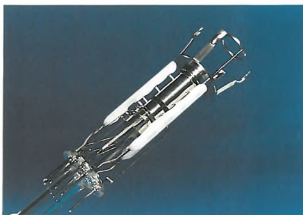
Fig. 10. The new design for the electron gun.
