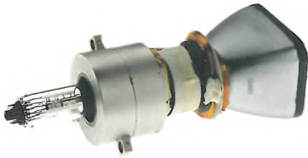
Fig. 11. Cathode-ray tube with the electron gun of fig. 10. The length of the tube is about 300 mm; the neck diameter is 36 mm and the screen diagonal is 125 mm.
