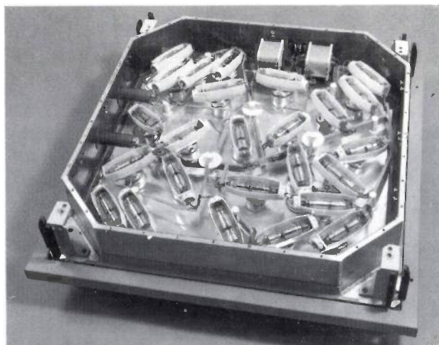
Fig. 5. An array of 25 small X-ray tubes whose focal spots are arranged in a non-redundant point distribution.
