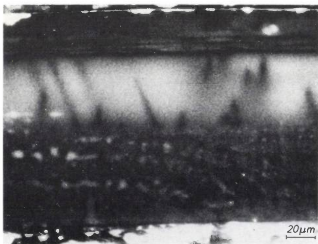
Fig. 4. Cathodoluminescence image, obtained with a scanning electron microscope, of an epitaxial GaP layer on a GaP substrate. The dark lines in the lighter part of the image indicate the presence of line dislocations in the epitaxial layer. This photograph was made by J. H. T. Hengst.
