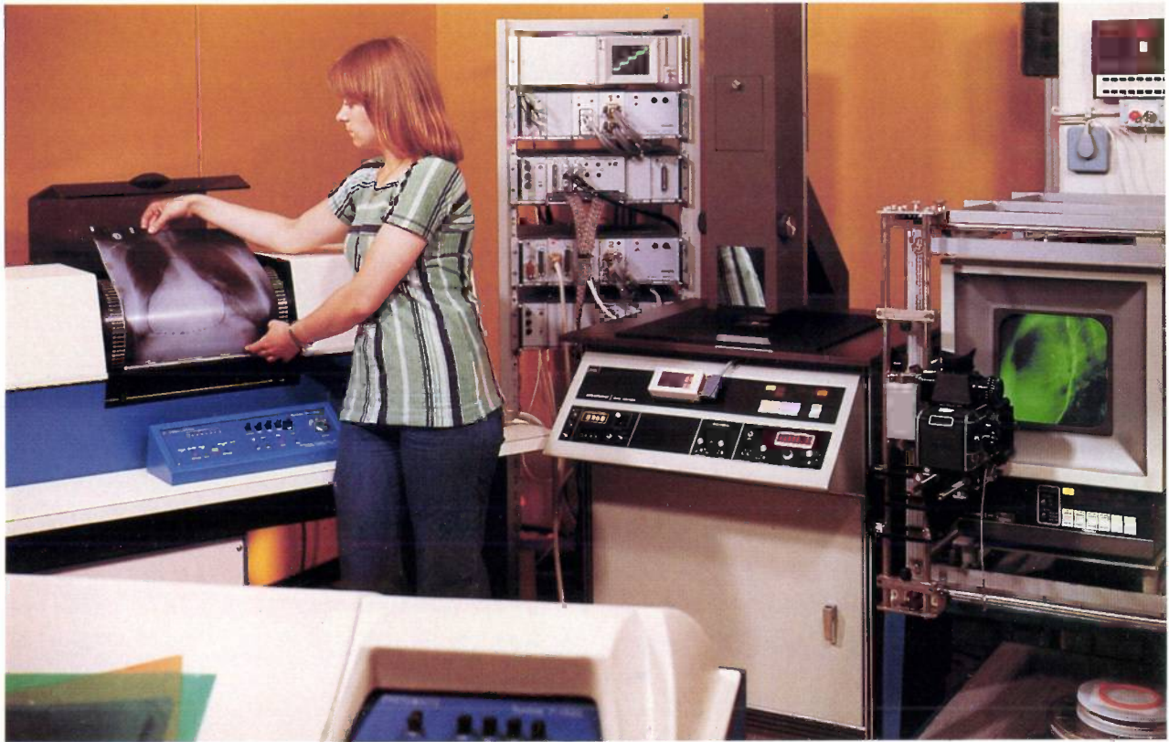
Fig. 2. This photograph shows part of the input and output equipment ( I and O , fig. 1, see also Table I). The operator is handling a picture intended for the drum photoscanner, which processes the larger formats (up to 350 \times 430 mm). The cover of the scanner has been moved back to show the drum on which the picture is mounted. The smaller formats (up to 57 \times 57 mm) can be digitized with the flying-spot scanner, the equipment near the centre of this photograph. The tall rack contains power supplies, interfaces for peripheral units and various control circuits. The small monitor screen at the top of the rack indicates the total range of brightness values present in the unprocessed image for the flying-spot scanner; by modifying the illuminance of the scanning beam this total range can be adjusted, so that it just matches the range of the detector (a photomultiplier). The large screen ( 177 \times 177 mm) on the right belongs to the output display unit. The output equipment in the foreground (only partly visible) provides film copies of the output image.
