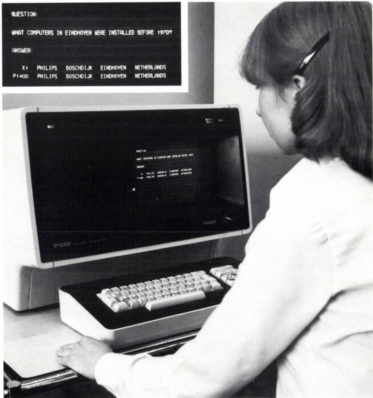
Fig. 1. The user of the PHLIQA 1 question-answering system simply has to type in his question in natural English. The answer 'computed' by the system appears on the display screen, which continues to show the question.
