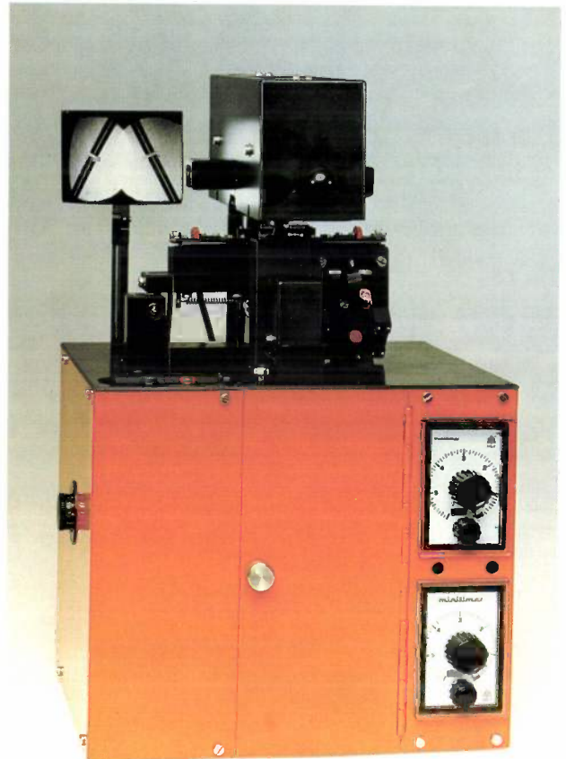
Fig. 1. The machine for hot splicing glass fibres for optical communication. The supports for the fibres (see also fig. 2), the positioning controls and the arc-discharge unit are all mounted on the cabinet. Above these there is a lamp housing, which contains two halogen lamps and optical components that project a 'stereogram' at about 60\times magnification on the screen at the left. The lamp housing can be swung aside to allow fibres to be inserted or removed. A safety switch then disconnects the high voltage from the arc electrodes. The positioning unit is operated manually: longitudinal displacements are controlled by two knobs below the lamp housing; radial displacements are controlled by the two small levers of a micromanipulator (the red knobs on the right). The cabinet contains the electrical components and a motor for the movement of the arc electrodes and for the automatic longitudinal displacement of the left-hand fibre during the splicing operation. This is preset by the knob on the left-hand side of the cabinet. The splicing time is preset by the time switch at the upper right. A delay between the preheating and the splicing operation can be introduced if necessary by means of the lower right-hand control. The green button at the left on top of the cabinet starts the automatic operations; the red knob on its right can be used to interrupt the procedure if necessary. The unit is 33 cm high and operates from a 220 V a.c. mains supply. The arc current is 13.5 mA d.c. at a voltage of 2600 V.
