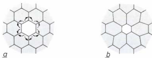
Fig. 15. Two forms of relaxation in a vacancy. a) Charge transfer. b) Transfer and deformation of the neighbouring atoms resulting in a cavity that is smaller than the free atom. These effects could explain a difference of about 20% between a_2 and a_1 but the difference is much greater than this ( a_2 \approx \frac{1}{3}a_1 ).
