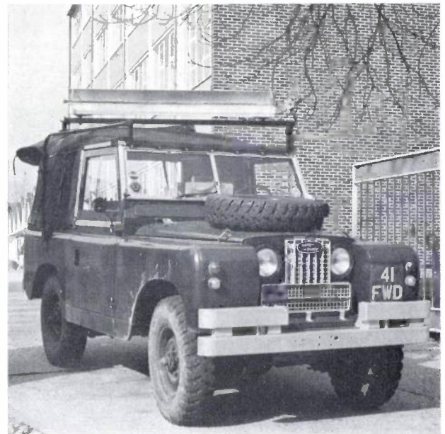
Fig. 4. The aerial mounted on top of a vehicle. The waveguide in the focal line of the parabolic cylindrical reflector can clearly be seen. The energy is fed in at the right and the fraction not radiated is absorbed in a load at the left. The portable television receiver for the display can be seen next to the steering wheel.
