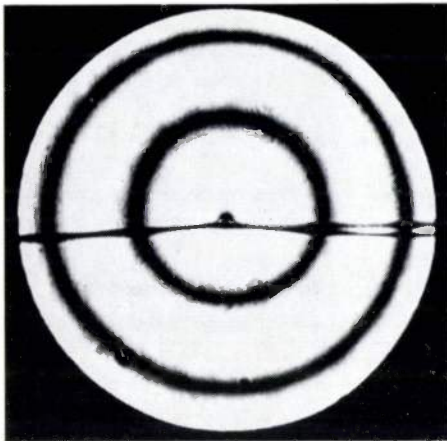
Fig. 4. Interference patterns in an axially symmetric argon-filled lamp (diameter of tube 4 cm; diameter of wire 200 \mu m) viewed along the filament. In this lamp each fringe order represents an isotherm. The effect of pressure variation at a constant filament temperature (1400 K) is demonstrated. In the tables m is the dark fringe order, counted from the centre.
