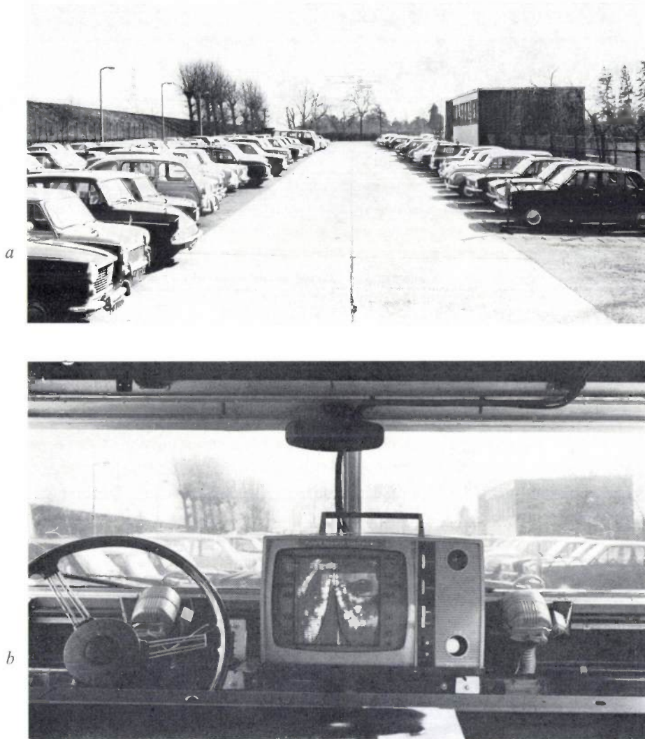
Fig. 7. a ) View of a car park. b ) The corresponding radar picture on the display in the vehicle. In front of the display screen there is a graticule giving a range scale and two converging lines indicating the free space required in front of the vehicle.
