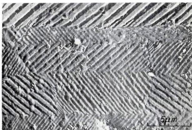
Fig. 12. Electron-photomicrograph of an etched surface of coarse-grained ceramic barium titanate. (After G. H. Jonker and W. Noorlander [21] .) The domain pattern, in which neighbouring domains differ from one another in their direction of polarization by 90^\circ , shows up because there is a difference in etching speed between the positive and negative sides of a domain.
