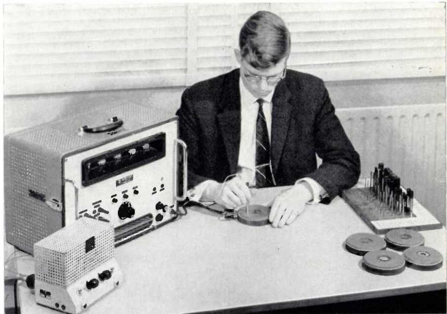
Fig. 4. Set-up for measuring the performance time for pin mounting (sticking a peg in a hole). The time taken for the operation is measured by the electronic counter on the left of the subject. This counter is set into action as soon as the pin leaves the starting circle (thus breaking an electric circuit), and counts the number of hundredths of a second which elapse before the pin reaches the bottom of the hole (when contact is restored). In order to obtain a sufficiently reliable average, the assembly operation was carried out 100 times for each pin. On the right-hand end of the table can be seen a number of plates with holes of different diameters, and pins which fit into the various holes with different tolerances.
