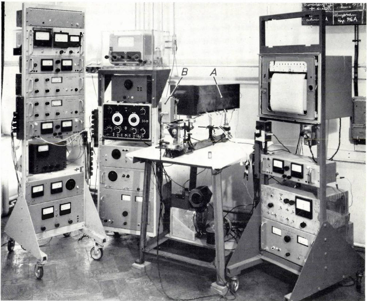
Fig. 2. Measuring set-up as in the diagram shown in fig. 1, used in the Philips Research Laboratories. The spot on the screen is scanned by slightly deflecting the beam. The testing tube is enclosed in a magnetically screened can of mu-metal ( A ). The photomultiplier is at B . The light-intensity distribution in the spot is approximately Gaussian (see the recording).
