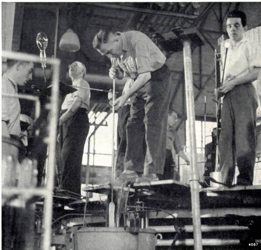
Fig. 2. Glass-blowers at work. The man on the right has just made a “gather” and has started to form the parison. The man in the centre (foreground) has completed the parison and is about to close the blow-mould (with a pedal). The third is inspecting a product fresh from the mould. The workman on the left removes the bulbs from the blowpipes. Between the first two glass-blowers (foreground) is a table for the rolling operation.
