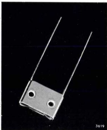
Fig. 7. The Mullard photoconductive cell ORP 10. The InSb element is visible on the edge of the drilled copper block. The leads to the InSb run through the copper block which thus serves as a heat sink during the soldering of connections.
