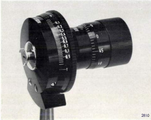
Fig. 16. Variable impedance as in fig. 15 , for 2 mm waves. The modulus and argument of the reflection coefficient can be read from separate scales. If reflection losses are eliminated, the absolute error in the modulus reading is less than 0.05.
