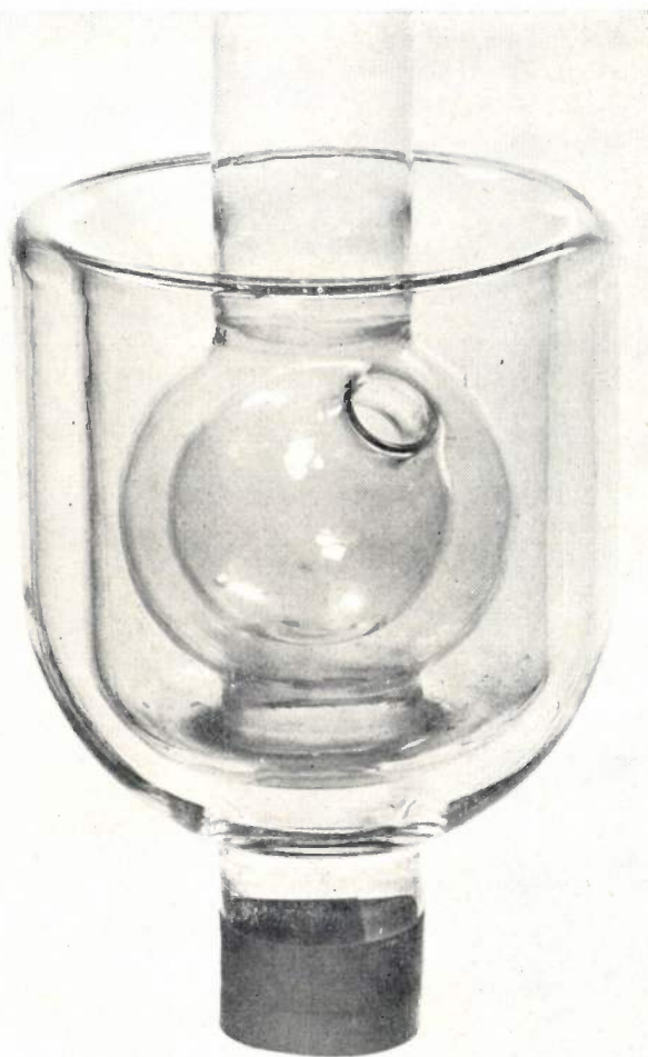
Fig. 13. Liquid-air-cooled vapour trap of very high conductance and high condensation efficiency, for an ultra-high vacuum pump built at Eindhoven (A. Venema and M. Bandringa, Philips tech. Rev. 20, 151, 1958/59). The vessel is filled by pouring liquid nitrogen (e.g.) into the "beaker"; the liquid then also enters and fills up the innermost bulb.
