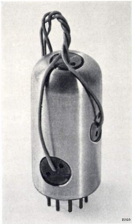
Fig. 2. Combination of three vibration pick-ups, used for measuring the vibrations to which tubes are subjected in electronic equipment. The whole assembly can be fitted in a tube holder in place of a tube.
