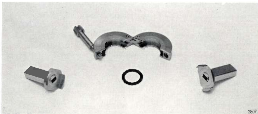
Fig. 9. Left and right, sections of waveguide with claw flanges; top centre, the hinged clamping ring which joins the flanges together; below, a rubber ring. (True size.) The clamping ring is tightened round the flanges with a single screw, perpendicular to the axis of the waveguide. The rubber ring ensures an airtight seal; the air in the whole waveguide system can then be put under pressure to prevent the entry of moisture.
