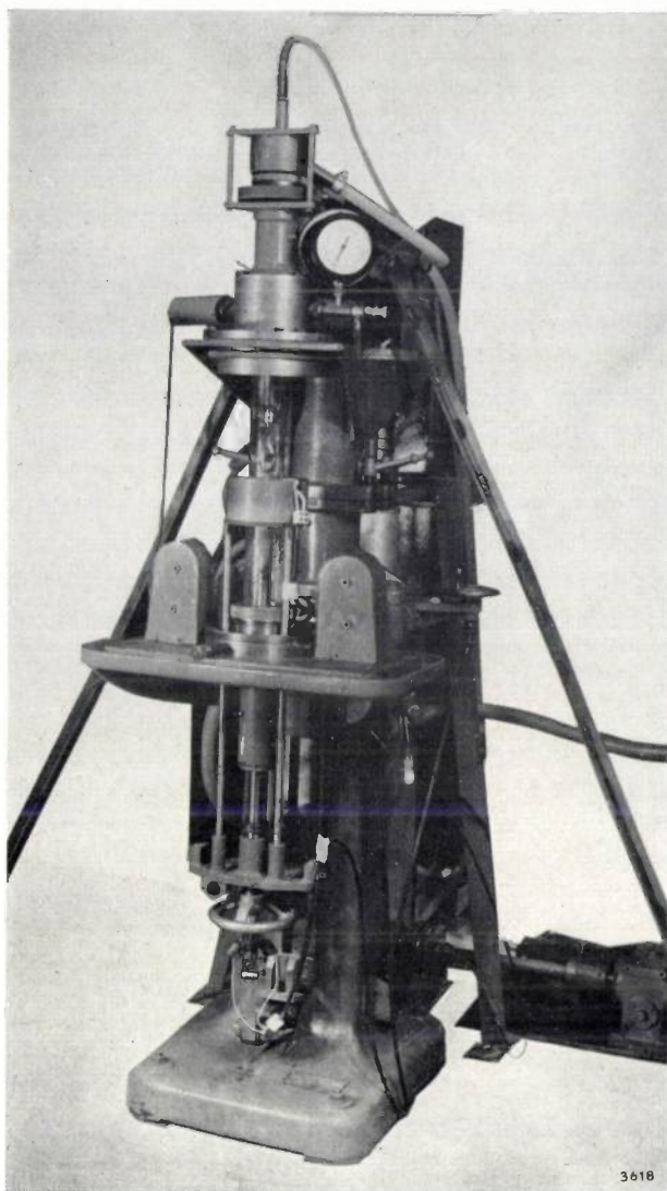
Fig. 5. Crystal puller used for production of single crystal InSb. The crucible is heated by radiation from a resistance coil not in contact with the crucible.
