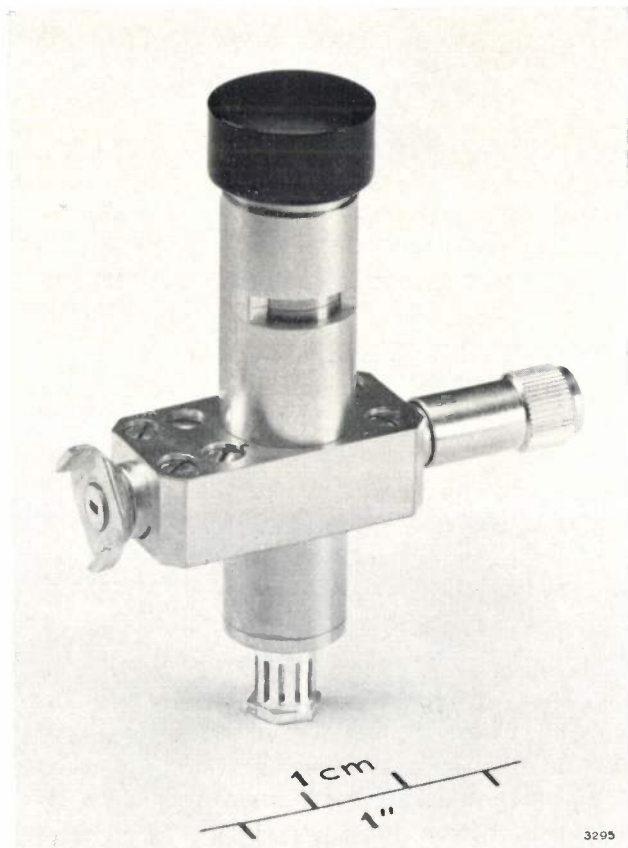
Fig. 1. Crystal detector for 2 mm waves. Left, claw flange, right, shorting plunger. The differential screw which is used to bring the silicon crystal into contact with the catswhisker is situated beneath the black cap; the displacement can be monitored through the window. Below: the coaxial connection for the millivoltmeter. The sensitivity is better than 10 mV per mW.
