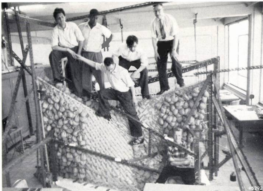
Fig. 14. The plywood model severely overloaded.
