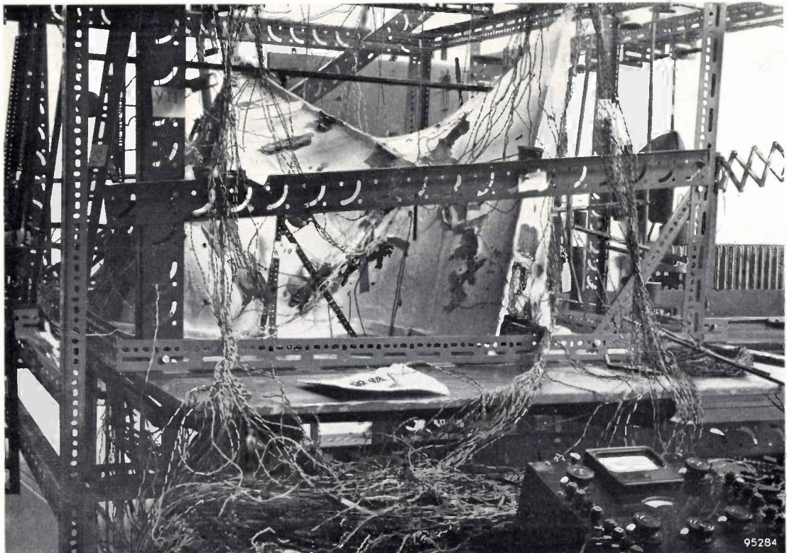
Fig. 4. Equipment used for measurements on the plaster model. A series of displacement dial-gauges are mounted on angle struts and connected via long rods to the model (shown more clearly in fig. 3 above). A large number of strain gauges are fixed to the shell surfaces and the ribs for determining the stresses (whence the elaborate wiring). Some of the indicating instruments are visible in the foreground.
