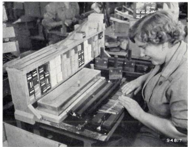
Fig. 4. Preparation of "thin" components having connecting leads. The leads of 50 or 100 components in a row are simultaneously bent over a jig so that they fit into the holes in the panel.
