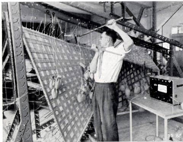
Fig. 10. Prestressing the plywood model.
