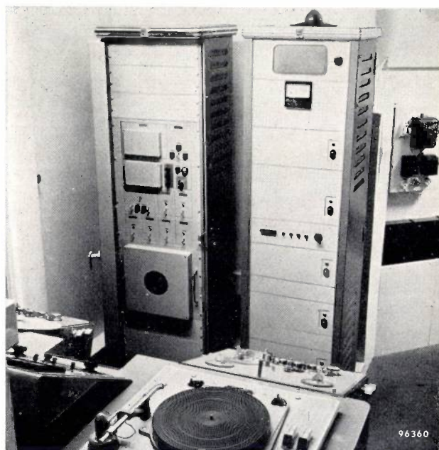
Fig. 23. Ambiophonic installation EL 6910 (left background) in the acoustic control room in the Palais de Chaillot. The reverberation time, and in each channel the loudness and timbre of the sound, can be adjusted either on the apparatus itself or remotely from a central mixing and control desk. The amplifiers are fitted with "Special Quality" tubes and have a frequency characteristic which is flat to within 1 dB from 160 to 12 000 c/s for 3 m/sec peripheral speed of the delay wheel and from 80 to 8000 c/s for 1.5 m/sec.
