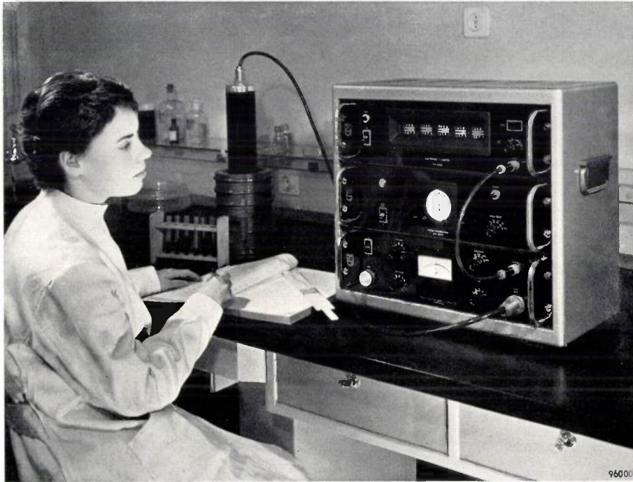
Fig. 3. The Philips scintillation counter in use. The upper part of the probe projects above a lead shield ("castle") at the bottom of which the radioactive specimen is situated. The probe is connected by a cable to the cabinet containing the rest of the electronic equipment. The bottom unit contains on the left the power pack for the photomultiplier tube (and to which a Geiger counter can also be connected) and on the right the pulse amplifier. The top unit contains the counting circuit, which also functions as pulse-height discriminator. The middle panel is fitted with a clock which indicates the time in which the apparatus has counted a pre-determined number of pulses.
