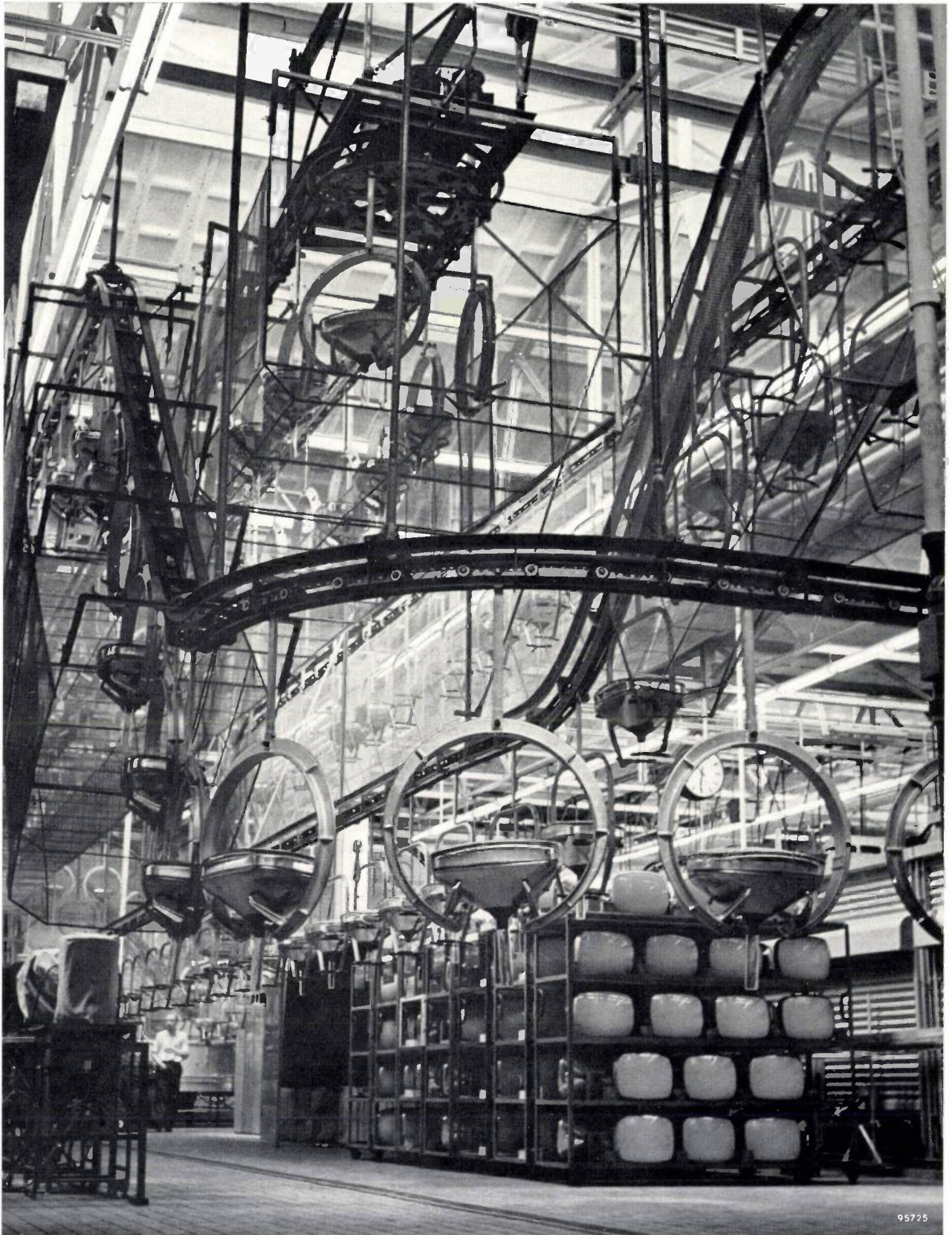
Transport system for 21 inch picture-tubes in the television tube factory of Valvo G.m.b.H., Achen.
