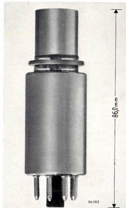
Fig. 4. The disc-seal triode EC 59. From top to bottom: anode bush, grid disc with screw-thread, cathode bush and pins in glass base. Through the glass spacer rings the actual electrodes can be seen.
