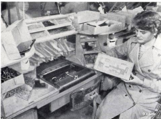
Fig. 5. Cutting and bending machine. a) A panel M is placed in the machine and the "thin" components inserted in the panel. b) The cover plate is closed, after which the machine automatically cuts and bends the connecting leads.
