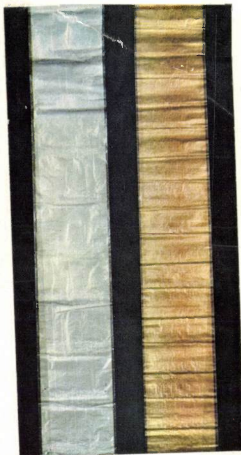
Fig. 2. Two strips of paper unwound from a capacitor which was switched off just before thermal instability would have caused breakdown. Left, a strip from the outside (coldest) layers; right, a strip from the inside (hottest) layers. The right strip has turned brown due to overheating.
