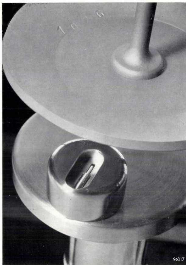
Fig. 1. Electrode system of an X-ray tube with rotating anode (the tungsten disc in the upper part of the photograph) and a double focus. This is a simple two-electrode system. The cathode here has two separate cylindrical filaments, the smaller one producing an extremely narrow line focus (width 0.3 mm).
