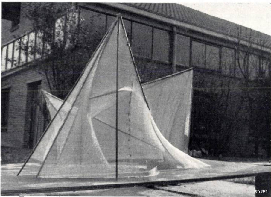
Fig. 1. Framework of tubes and wire-gauze for making the plaster model of Philips pavilion, scale 1 : 25 (T.N.O. Institute, Rijswijk, Netherlands).
