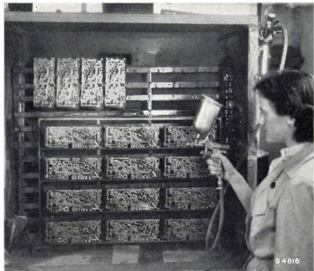
Fig. 3. Spraying soldering flux on the printed wiring.
