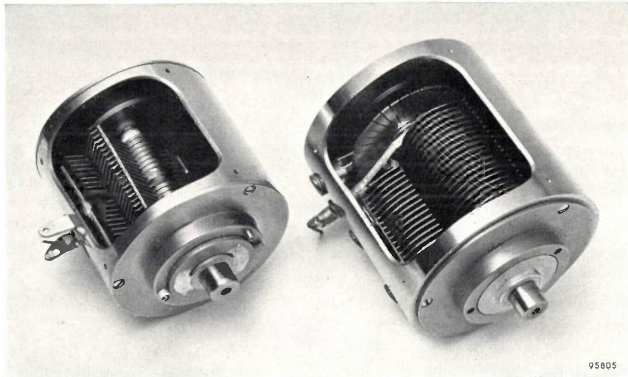
Fig. 1. The two precision capacitors with covers removed. Left, the linear-law capacitor. Right, the sine-law capacitor.
