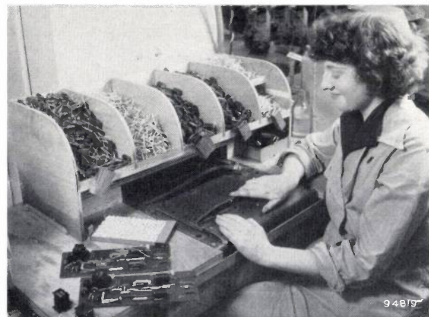
Fig. 5. Cutting and bending machine. a) A panel M is placed in the machine and the "thin" components inserted in the panel. b) The cover plate is closed, after which the machine automatically cuts and bends the connecting leads.
