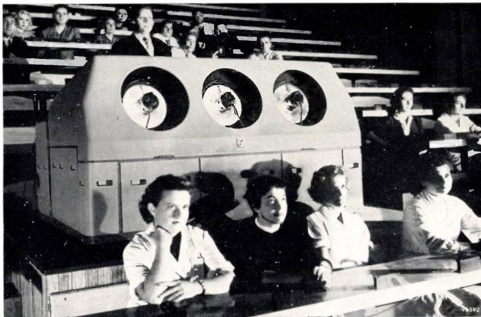
Fig. 4. The colour-television projector in the lecture theatre. The primary-colour projectors (red, green, blue) are mounted side by side 5 ).
