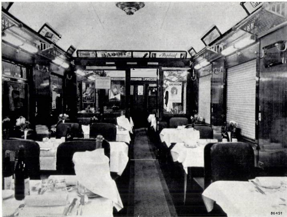
Fig. 6. A restaurant car of the Compagnie Internationale des Wagons-Lits, lit with 15 W "TL" C lamps.
