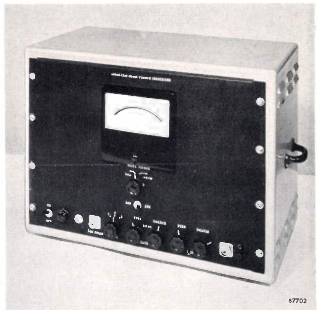
Fig. 3. Automatic noise factor indicator constructed in accordance with the block diagram of fig. 2. (The instrument is not being manufactured.)
