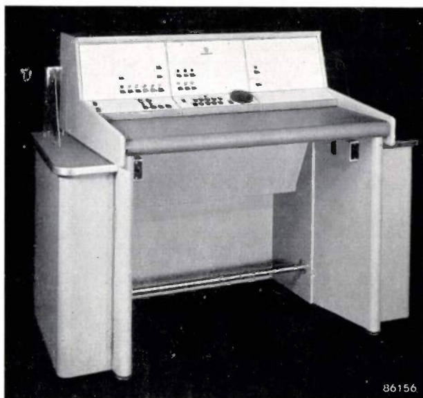
Fig. 8. Operators desk for handling the local traffic of a PABX type UB 49 with an arbitrary number of public lines.
