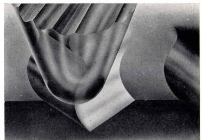
Fig. 4. Perspective drawing, showing the static situation with the stylus resting in a modulated groove.
