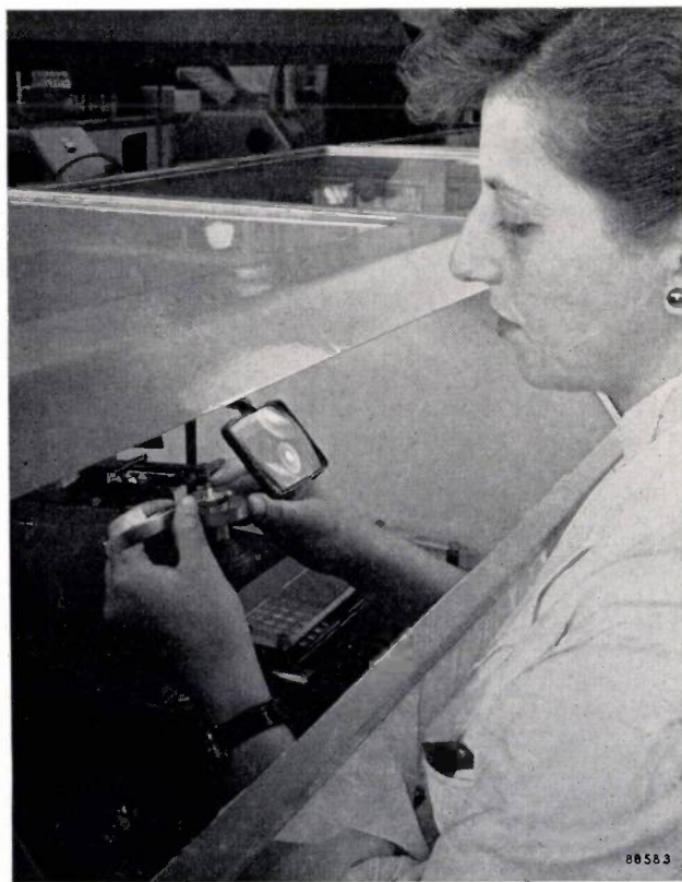
Fig. 5a. Assembling the electrode system of an amplifier valve. This operation, like that in fig. 5b , is carried out under a transparent dust-cover. The operator's hands enter the dust-cover through slits in a nylon curtain, which produces no dust itself.
