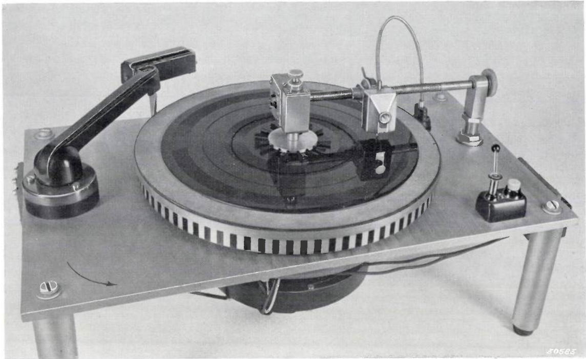
Fig. 4. The recorder in action. At the centre and outer edge of the record, shorter recordings have already been made. The shaving from the grooves just cut may be seen lying on the record in a circle slightly smaller than the groove (normally the shaving is removed by the brushes at the centre). On the left, the pick-up for reproduction. Right foreground the switch. Along the circumference of the turn-table may be seen the divisions which serve for checking the number of revolutions per minute. Under the turn-table the motor is suspended on springs.
