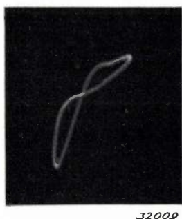
Fig. 7. Unsymmetrical oscillogram such as is obtained at an arbitrary direct voltage in the neighbourhood of a potential jump.
