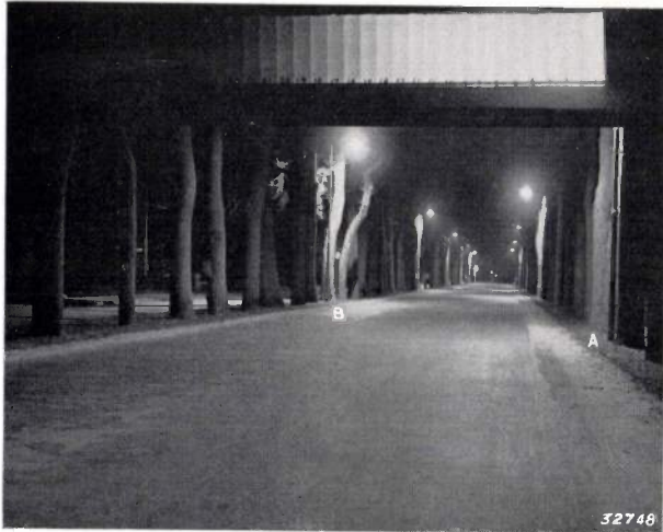
Fig. 5. Photograph of the road Vught-Tilburg used for the measurement of the distribution of brightness given in fig. 6. The observer (the camera) is situated on the line QQ in fig. 1 at such a point that the black stripes bound the part of the road lying between 23 and 63 m from the observer. In this section the distribution of brightness was measured. At the top may be seen the density marks used.
