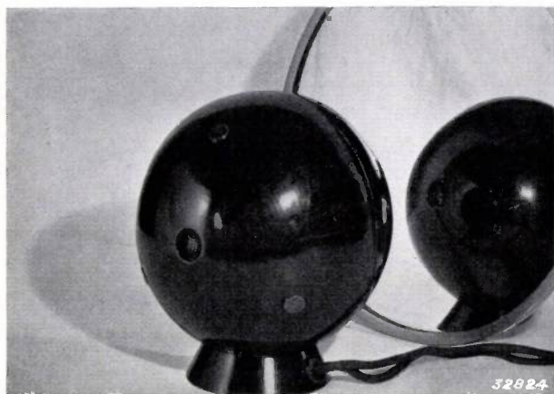
Fig. 4. The sphere used as "artificial head". It has a diameter of about 22 cm. The two microphones are mounted at the extremities of a horizontal diameter. (In order to make visible both microphones the sphere has been placed before a mirror.)
