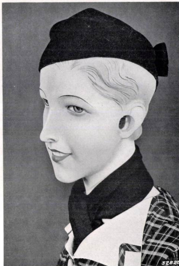
Fig. 5. The model with which the influence of the details of the shape of the head were studied. The microphones are mounted in the ears and feed the head-phones of the user.
