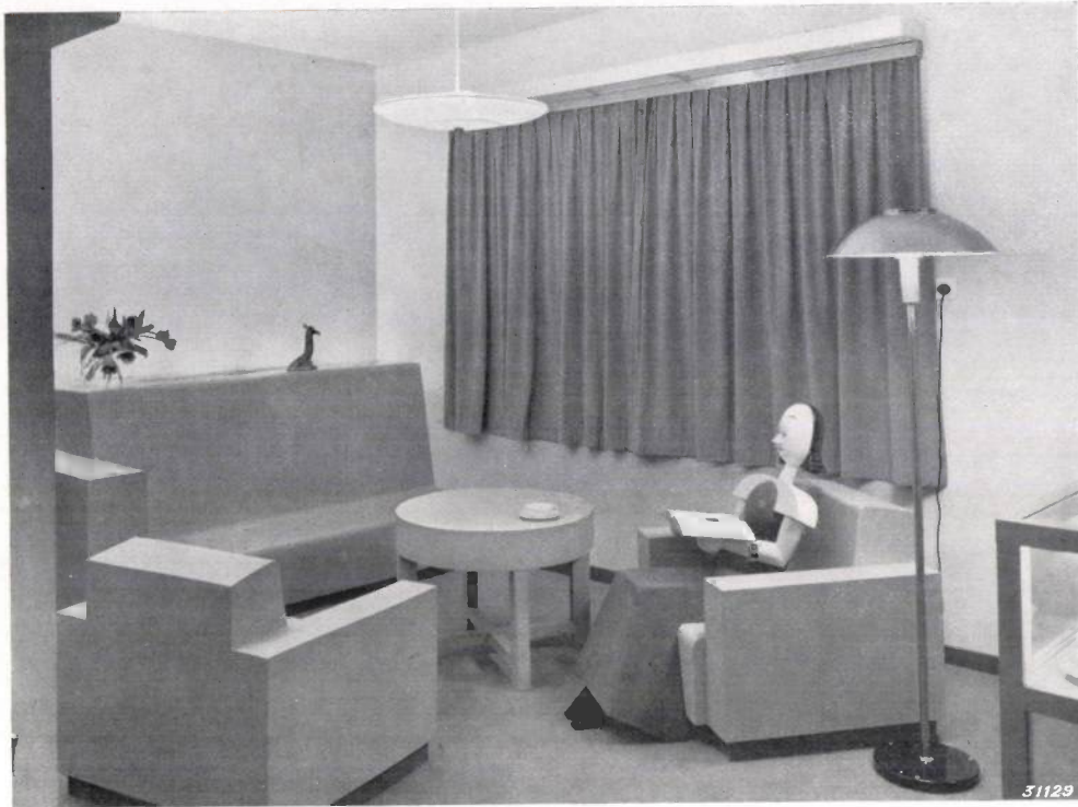
Fig. 5. Living room. General semi-indirect illumination by a central ornament made of parchment, 3 lamps of 100 Dlm (Dlm = dekalumen = 10 lm). Local illumination for reading and sewing from a standard lamp "Philihome" 50 with a lamp of 200 Dlm, 150 W. Intensity of illumination on the reading matter 300 lux. A wall illumination behind the couch decreases the contrasts in the room.
