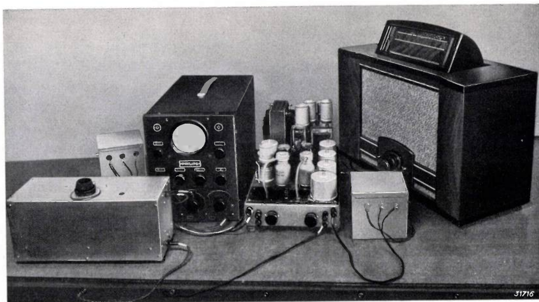
Fig. 2. Photograph of the complete apparatus. To the left the oscillator, behind it the filter for removing the harmonics. In the middle of the screen of the cathode ray oscillograph the semi-circle may be seen. To the right beside the oscillograph is the amplifier with the phase rotating circuit (4 and 5 of fig. 1), and the filter for the music voltage; on the extreme right the radio receiving set.
