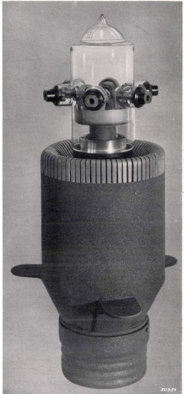
Fig. 3. The transmitting valve PA 12/15 surrounded by a cooler through which a current of air is sent from bottom to top.
