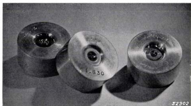
Fig. 7. Dies with a core of "hard cemented carbide".
