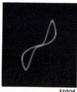
Fig. 10. Symmetrical oscillogram recorded with too high an alternating voltage.
