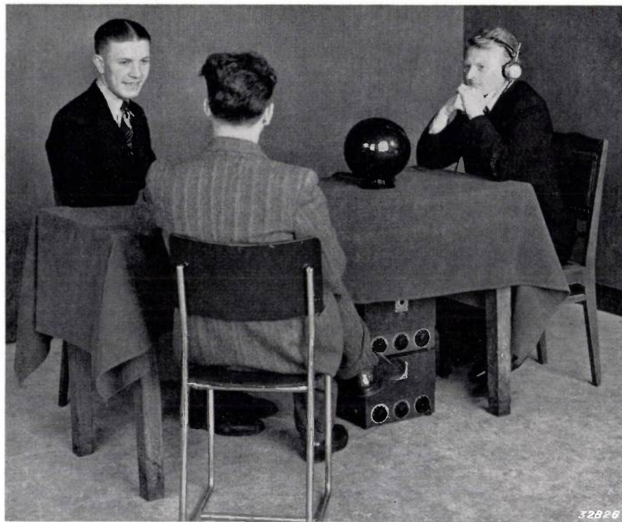
Fig. 6. View of the apparatus during use. The artificial head is placed on the table. The two amplifiers are set up under the table.
