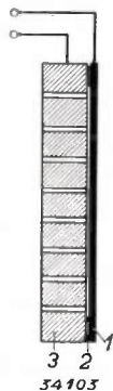
Fig. 1. Diagram of a condenser microphone. The membrane 1 is placed at a very small distance (16 \mu ) from the rigid plate 3. The separation is determined by the thickness of the ring 2 lying between 1 and 3 together form a condenser whose capacity varies upon vibration of the membrane. With constant charge voltage variations hereby occur between 1 and 3, which after amplification may be measured. Plate 3 is provided with a number of holes in order to prevent the rigidity of the cushion of air between 1 and 3 decreasing the sensitivity of the microphone.
