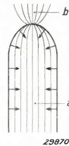
Fig. 3. Current lines of force at the top of the welding rod. The arrows indicate the direction of the electrodynamic forces. The convergence of the current lines gives rise to a resultant downward force.
