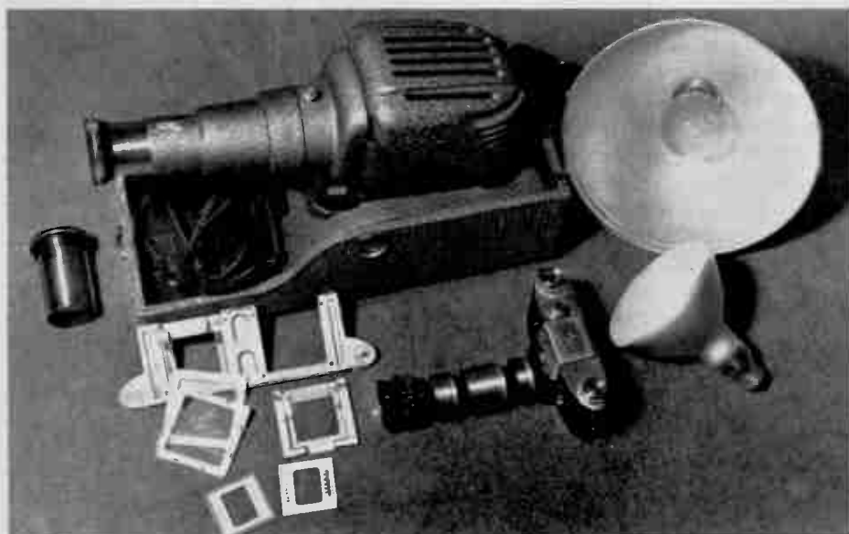
Figure 2. Basic Equipment Used for Making and Projecting Slides. (The projector shown can handle either 2'' \times 2'' or 2\frac{1}{4}'' \times 2\frac{1}{4}'' slides. The camera is equipped with extension tubes, which allow the making of close-ups. Two types of flood lamps are shown, one with a metal reflector and the other with a built-in reflector.)
