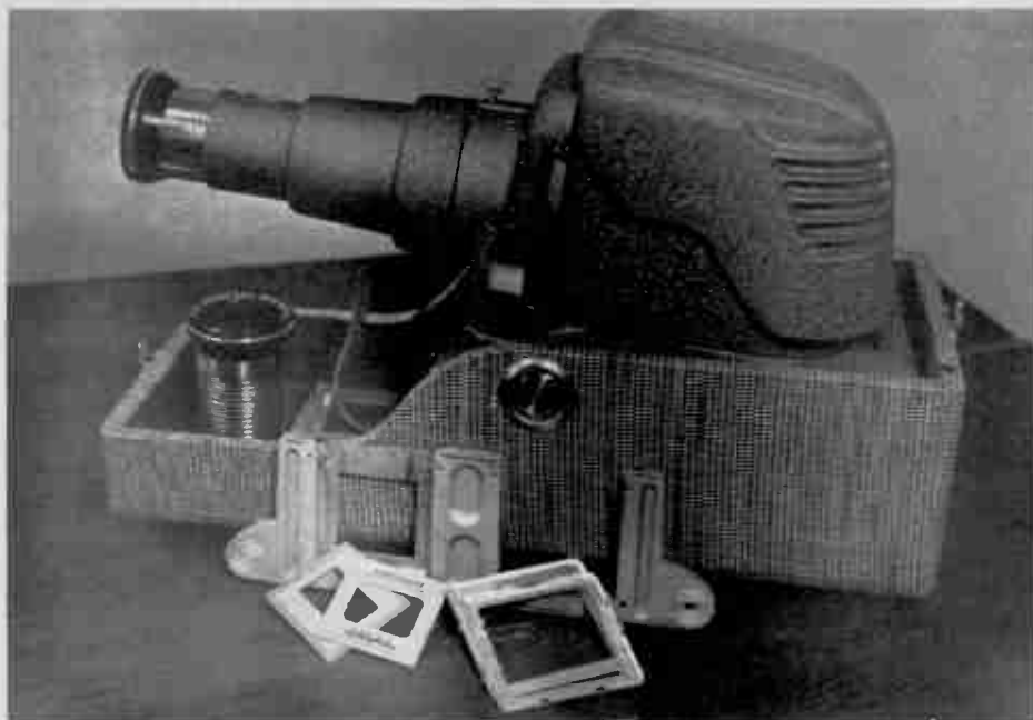
Figure 1. Example of a Typical Slide Projector. (The additional lens has a different focal length, and, while not necessary it will give the advantage of better control over projected-picture size. Examples of glass ( 2\frac{1}{4}'' \times 2\frac{1}{4}'' ) and cardboard ( 2'' \times 2'' ) mounts are shown. A choice of glass or cardboard is available in both sizes.)
