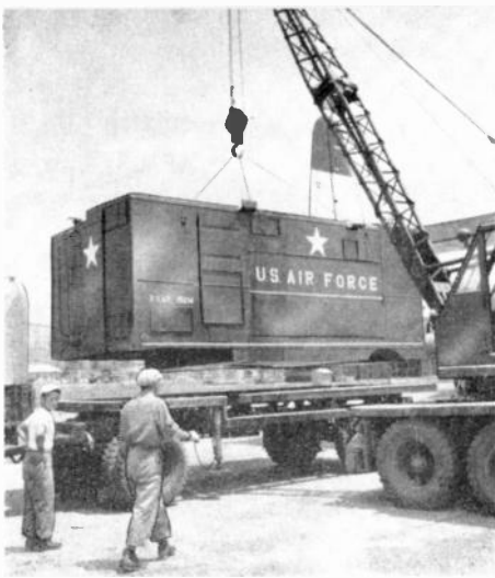
Figure 2. Body Being Lifted by Crane
