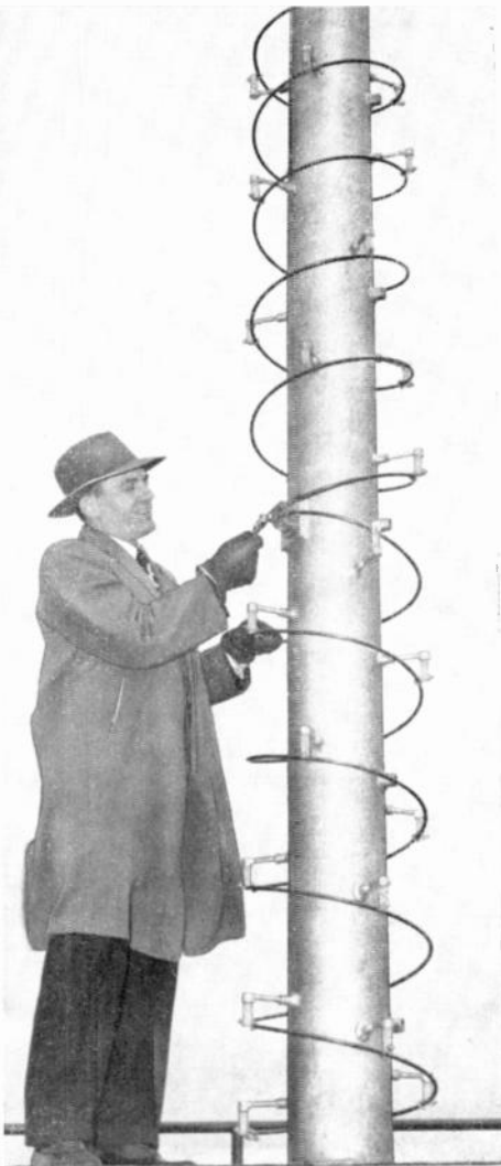
Figure 3. One Bay of a 500-Mc. Antenna ample, that a helical antenna with a power gain of 20 would have an equivalent power gain of about 22 if the vertical component were not present.
