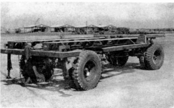
Figure 5. Trailer Chassis with Girders and Rear Pulley in Place
