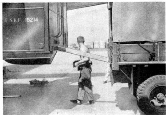
Figure 10. Prime Mover Pushes Unit Fully into Plane
