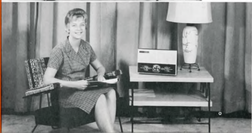
A particularly good program on Philco's twin-speaker Model 912 AM/FM set pleasantly interrupts the reading of Joan Wasikowski, Marketing. The set has seven tubes and a silicon rectifier; automatic frequency control with a transistorized circuit to guarantee no FM drift, vernier tuning, finished band shell back. It comes in beige and ivory and white and black.
