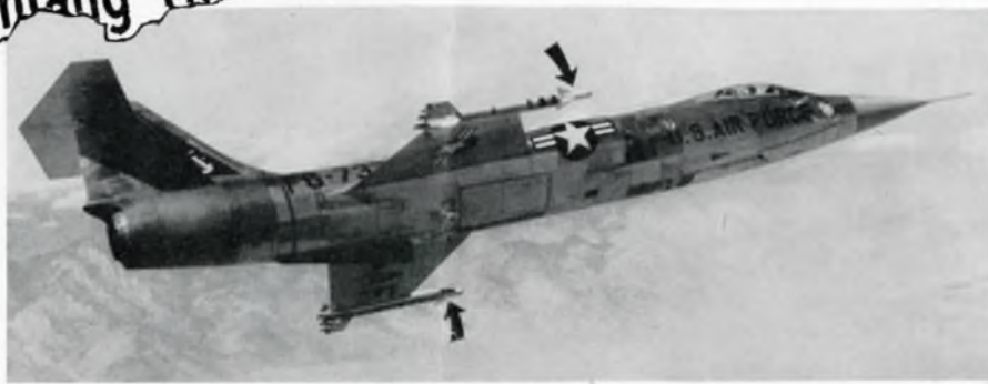
ARROWS POINT TO SIDEWINDER MISSILES ON WING TIPS OF F-104A STARFIGHTER
