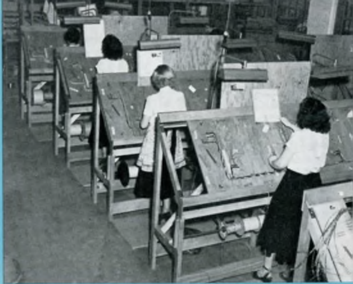
▲ THE CABLE fabrication section of Philco's microwave production at Plant 18 contains special cabling equipment developed by the Company to make possible a wide diversification of units.
