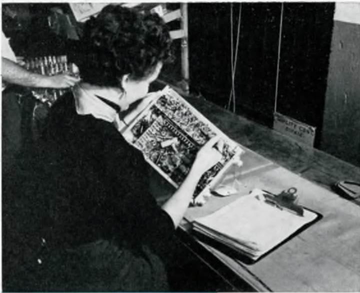
ONE OF THE MANY separate quality control tests is made on IF and Video chassis.
