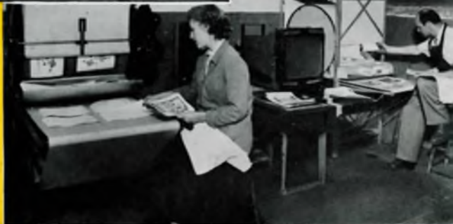
PHOTOGRAPHS are put ► through the rotating drum dryers at the left. In the center is the 11x14 camera.
