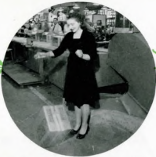
NOTHING TO WORRY ABOUT —Etta Lou Wright, Quality Control, drops a packaged radio receiving set to the concrete floor of Plant 2 . . . but it is for testing on the efficiency of the packaging, cabinet and chassis structure. Daily, Miss Wright removes current models from the radio production line for inspection as to their appearance, sensitivity, tone, selectivity, dial operation and distortion.
