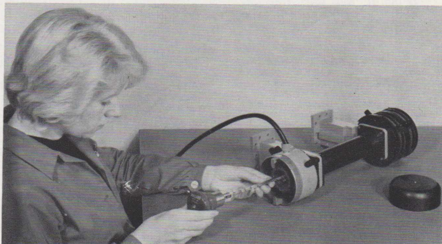
Operator mounting High Power Travelling Wave Tube type LB4-20 into mount type P4L-5.
