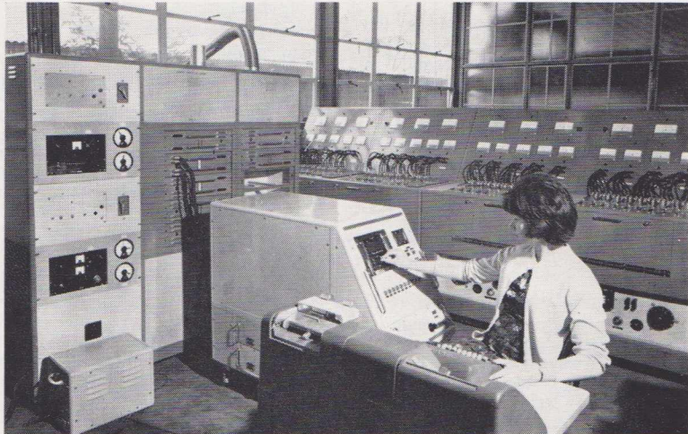
Transistor characteristics being automatically measured during life testing.
