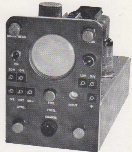
A typical, simple oscilloscope.
