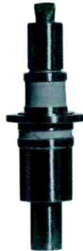
Figure 5 — Machlett ML-6771 — First Triode used in C-Band equipment. ML-6771 and its associated cavity, ACF Model 350, have successfully operated under tests to 30 g from 20 to 2000 cps.
