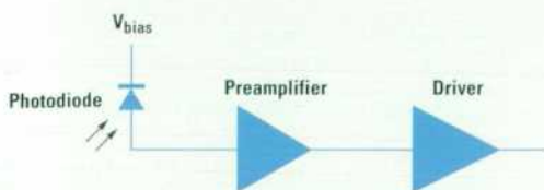
Fig. 1. Block diagram of amplified O/E converter.
