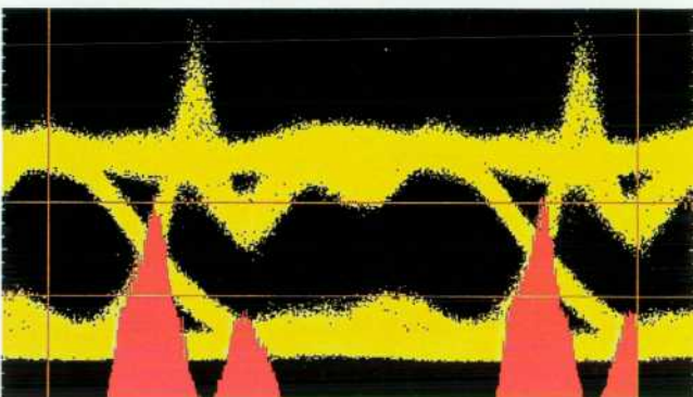
Fig. 6. Horizontal histograms are used to find the eye crossing times. The window is set to exclude the logic one and zero level data.
