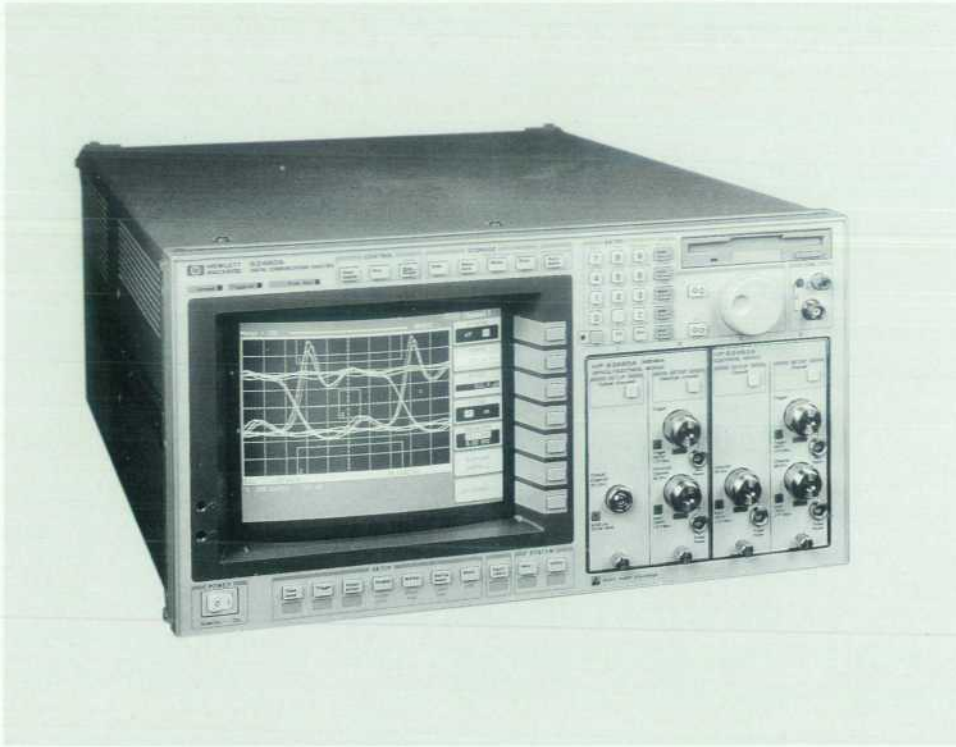
Fig. 2. The HP 83480 digital communications analyzer combines a SONET calibrated reference receiver with an oscilloscope and communications measurement firmware.
