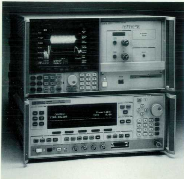
Fig. 4. Named for its ability to measure very fast magnitude and phase transitions under pulsed-RF conditions, the HP 71500A microwave transition analyzer (top instrument) is part high-frequency sampling oscilloscope, part dynamic signal analyzer, and part network analyzer. The HP 71500A consists of the HP 78020A microwave transition analyzer module and the HP 70004A mainframe. The bottom instrument shown here is the HP 83640A synthesized sweeper.
