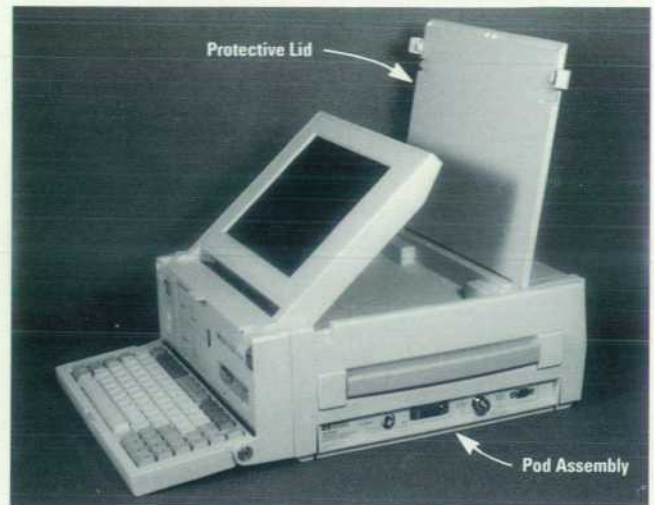
Fig. 4. The protective lid used to protect the display during travel. Also shown is the location of the detachable pod assembly which snaps into the underside of the mainframe of the Network Advisor. The pod assembly is discussed later in this article.
