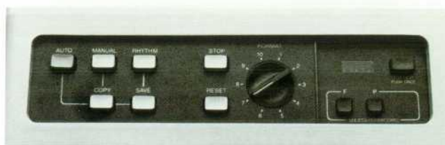
Fig. 6. Control panel of the 4700A. The recording function is selected by using the keys on the left and the format can be selected and/or modified by using the display, keys, and rotary switch on the right.
