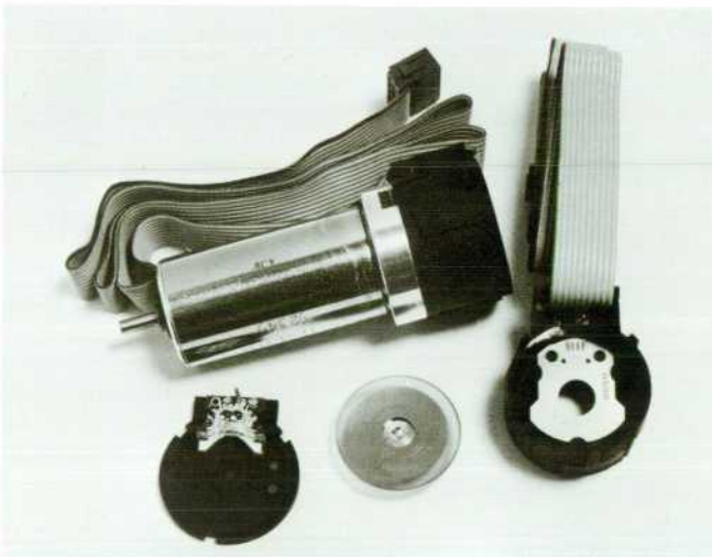
Fig. 1. The HP HEDS-5000 encoder Kit makes it easy to add the capability of sensing shaft position and velocity for digital control. The kit has three parts: an encoder body containing the phase plate and detector module, a code wheel assembly, and an endplate containing the emitter module.
