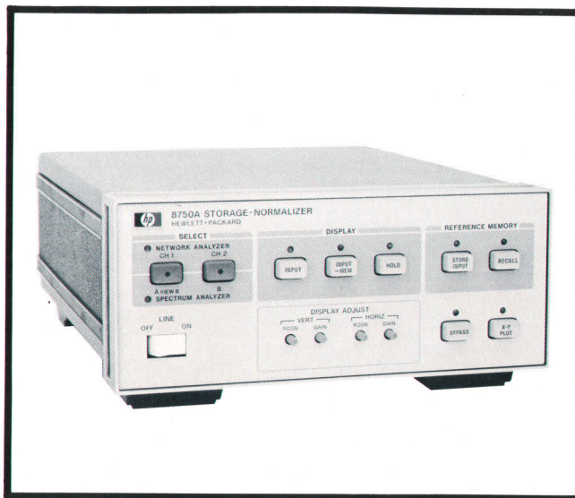
Fig. 3. Model 8750A Storage-Normalizer retains the results of dual-channel swept-frequency or other-type measurements for flicker-free display, normalization, and comparison. It works with suitably equipped frequency response sets and spectrum analyzers in HP 180-series mainframes and with the 8407A and 8410A/B Network Analyzers. It can work with spectrum analyzers in HP 140-series mainframes with the addition of a display monitor or oscilloscope. It also works with other types of instrumentation.
