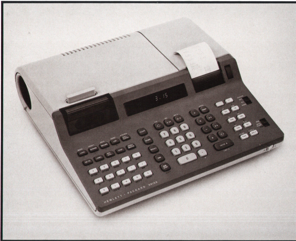
Fig. 1. Model 9815A Calculator includes as standard many formerly optional features, including printer, magnetic tape unit, and 15 special function keys. The keyboard language is reverse Polish. Memory is expandable from 472 program steps to 2008 program steps.
