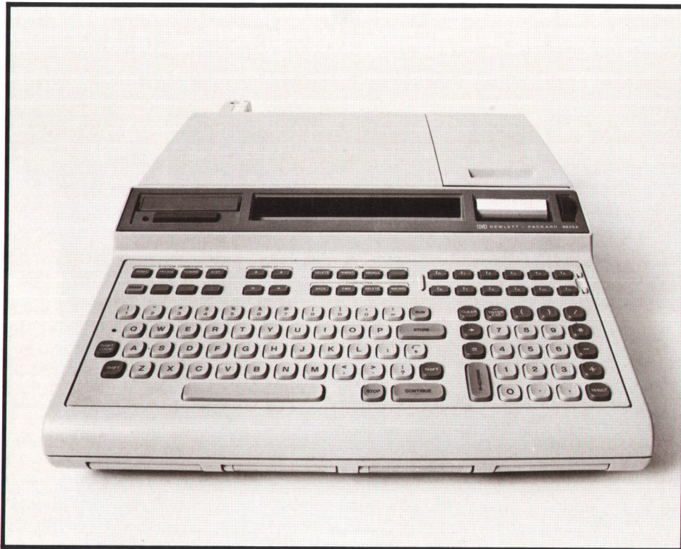
Fig. 1. Model 9825A Calculator can be used as a stand-alone programmable calculator or as a system controller. Major new features include two-level priority interrupt, direct memory access, live keyboard, multidimensional arrays, high-performance tape drive with automatic memory record and load capability, and extended internal calculation range. The keyboard layout is based on that of a standard typewriter with the addition of a number pad, system command and editing keys, and twelve user-definable keys. The programming language is called HPL.
