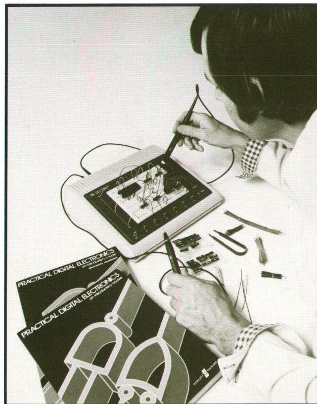
Fig. 1. Model 5035T Logic Lab includes everything needed to train newcomers to digital integrated circuits: hardware, textbook, laboratory workbook, and all parts and troubleshooting tools.
