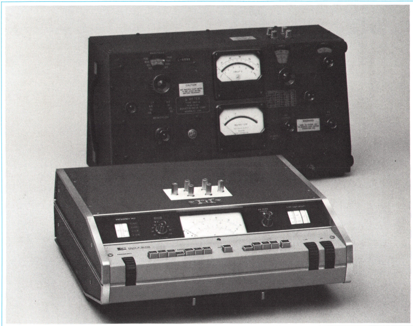
The classic Boonton Q Meter, now the HP Model 260A, has been redesigned with an extended Q range and circuit improvements that make it faster and easier to use.
