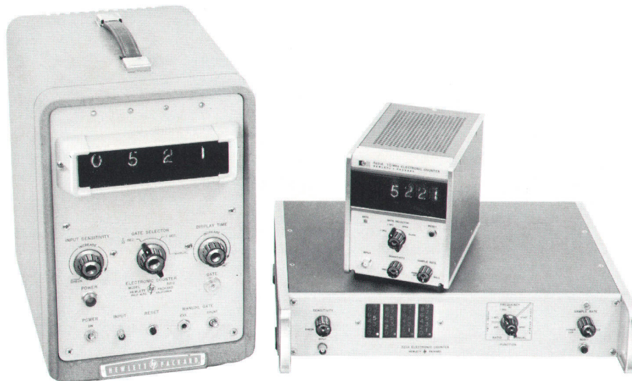
Fig. 1. Clockwise from left, HP Model 521A Vacuum-tube Counter, HP Model 5221A Integrated-circuit Counter, and HP Model 5211A Transistorized Counter. Counter specifications have steadily improved while prices and sizes have dropped.
