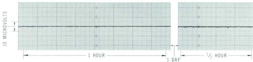
Fig. 3. Record showing typical stability achieved by new amplifier over long intervals under room conditions. Record made with new amplifier operated in high-gain position ( \times 1000 ) using M2 plug-
