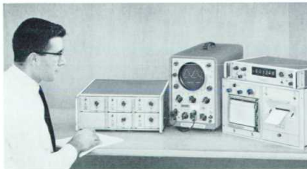
Fig. 1. New solid-state dc amplifiers (group of five in case at left) have high stability, low drift, fast recovery on large overloads, and use panel plug-in modules to adapt to many uses. Unit is produced by -hp-'s Dymec division.
