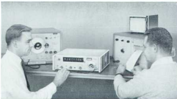
Fig. 1. New -hp- high-speed frequency counter (center) measures from 0 to 20 or 50 megacycles in two models, has accessory plug-ins to measure to 500 megacycles. Counters have very high stability time bases for high accuracy in demanding measurements. Counters can be used with many other data-handling devices.
