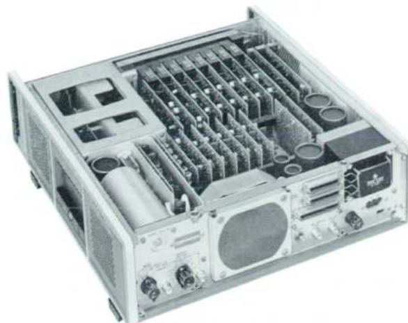
Fig. 12. Circuitry in counters is built up on removable computer-type circuit boards to achieve compact overall size and high accessibility.
