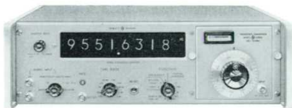
Fig. 4. New -hp- Model 5243L 0-20 Mc Counter with Model 5253A 100-512 Mc Converter plug-in.
