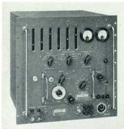
Fig. 2. Model 524B Counter with frequency converter plug-in unit in place.
