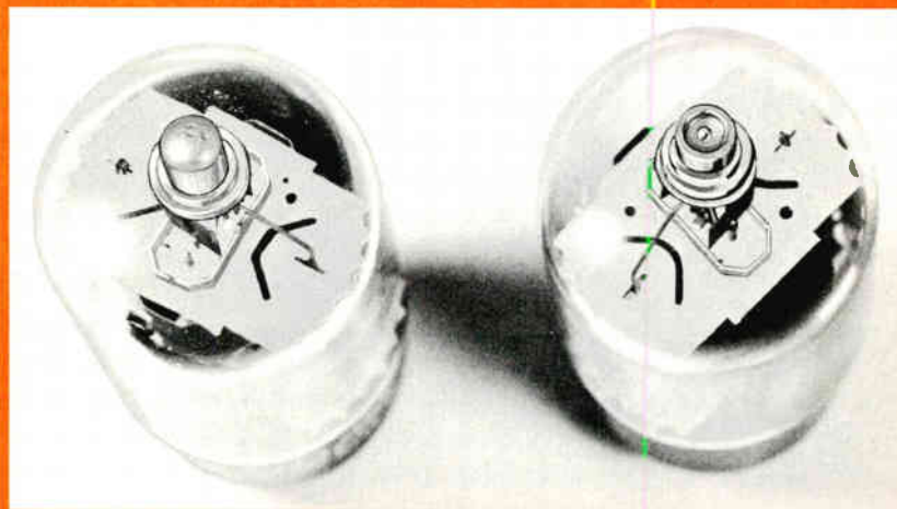
The top cap on the right is welded and does not require solder which could loosen due to heat build-up.
