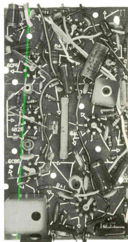
Fig. 1. Component side of I-F board used in "M-5" line of General Electric TV receivers.
