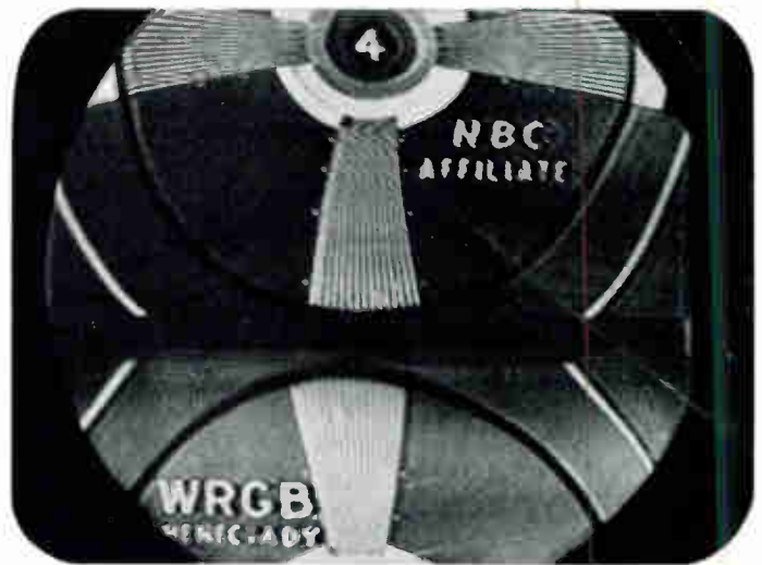
Tele-Clue No. C86. This is a somewhat unusual defect which could take a considerable amount of time to run down. The picture was very dark and looked as if the contrast control was advanced too far. This control however, had no noticeable effect on the picture. The horizontal sync was critical and the vertical would jump a frame quite frequently. This condition was caused by a leaky capacitor C290 in Fig. 2. Because of this a positive voltage (50 V.) appeared on the picture tube grid. This circuit was used in the following General Electric TV receivers:
