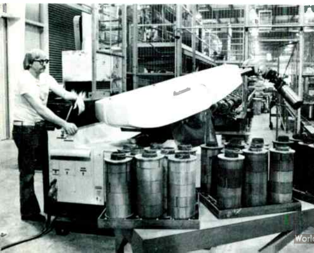
An industrial robot (l) lifts stator laminations at General Purpose Motor plant in Linton, Ind. Below: Meter plant robot used in die-casting at Somersworth, N.H.; and right, a spray-painting robot in Major Appliance facility at Cicero, Ill.
