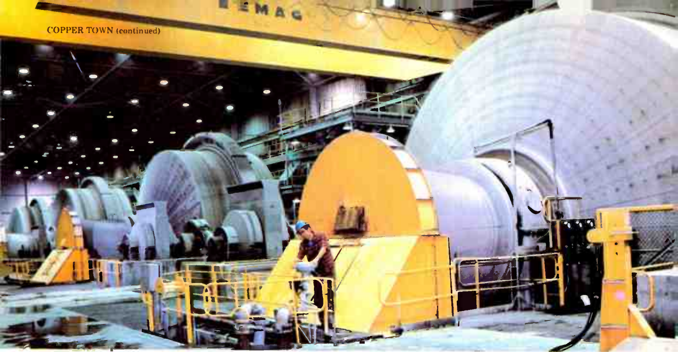
Canadian GE motors power the operation's six behemoth grinding mills.
