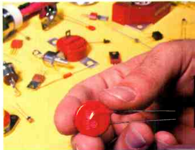
New GE-MOV® varistors, above, protect sensitive solid-state components against voltage surges. Integrated General Electric communications system (left) provides electronic efficiency for modern police and fire operations.
