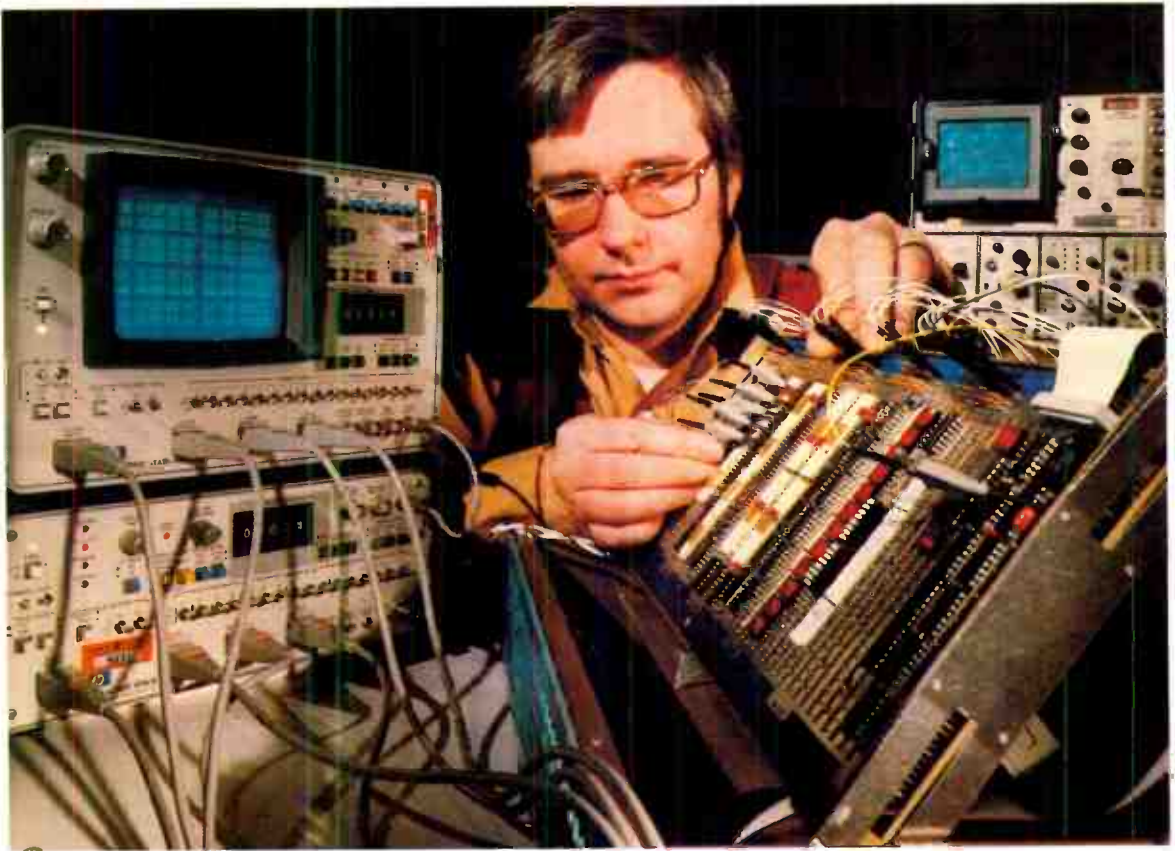
New microprocessor used to improve existing systems is checked on an "emulator" (above) in General Electric's Electronics Laboratory.
