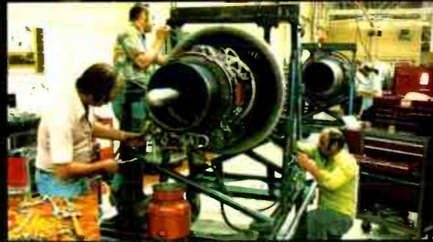
11:30 p.m.—In GE overhaul shop, N500PC's engines join others being reworked into "zero time" engines.
