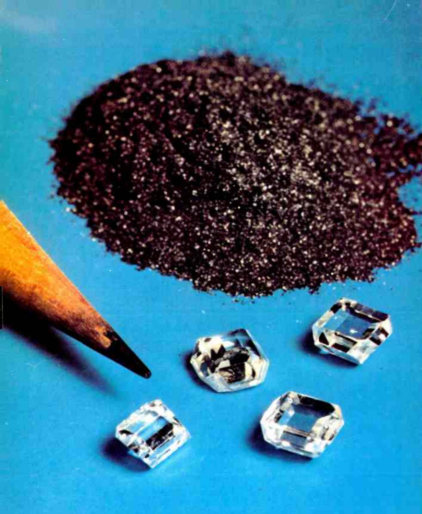
From dirty graphite to gem-quality diamonds—GE's Man-Made ® industrial diamond is one of the closest things to alchemy man has ever achieved.
