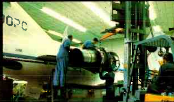
8:00 p.m.—N500PC's engines are lifted off the aircraft to begin their trip through GE's overhaul facility.
