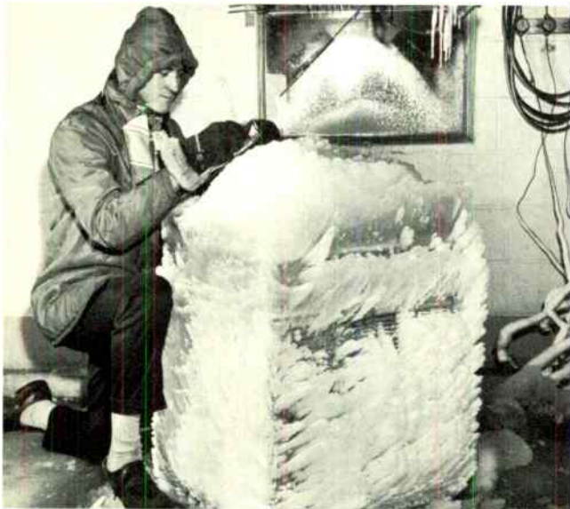
A "deep freeze" is one of the exhaustive laboratory tests that General Electric's Weathertron heat pumps must endure.
