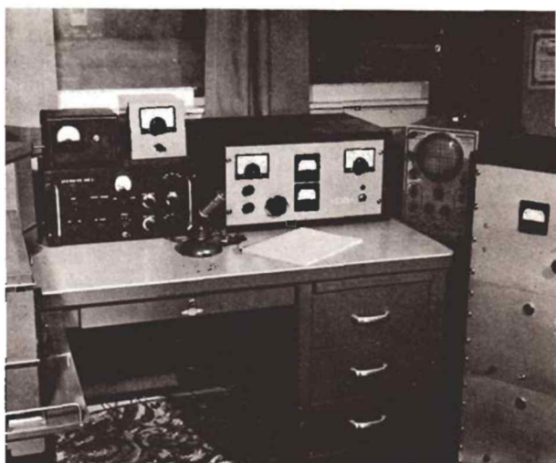
COMPLETE STATION at K2IOW with the Compact Triode Kilowatt at the right side of the operating desk. Other equipment includes an NC-240D receiver and speaker (extreme left); the 6L6-GC exciter which drives the 810 final; indicator for SWR bridge and High-C Bandswitching VFO atop the exciter; 5-inch 'scope for monitoring; and a 3-foot-high rack cabinet containing (top to bottom) class B GL-805 plate modulator, high voltage supply for the modulator, and a 2,000-volt DC supply for the 810 final.
