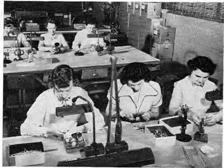
A portion of the Du Mont incoming parts inspection group. Thorough inspection of component parts minimizes rejection during subsequent tube testing
