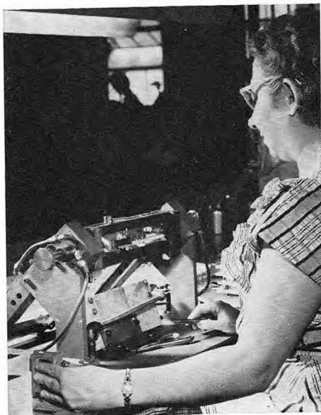
Glass-rodging portion of the electron-gun assembly utilizes a concise mechanized jig to prevent variables introduced by an operator. Heating and cooling of the glass rods is automatically timed. The position of the gun in the jig is also automatic
