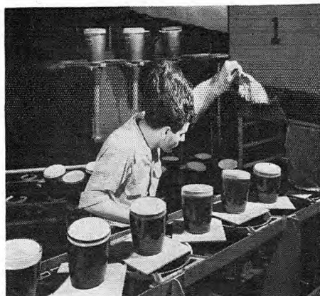
Screen baking operation thoroughly dehydrates the screen and is the first step in out-gassing the tube. All baking is done at precisely controlled temperatures to prevent change in spectral characteristics from tube to tube
