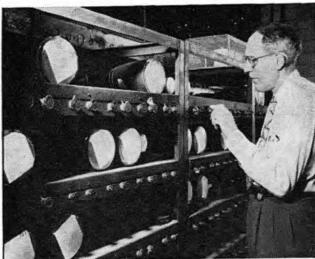
Tubes are given life tests of 500 hours, some for 1000 hours, and others to destruction. Shown giving the set-up a spot check is Mr. John Hinck, whose 22 years with Du Mont in the relatively new cathode-ray tube field is typical of the experience within the company
