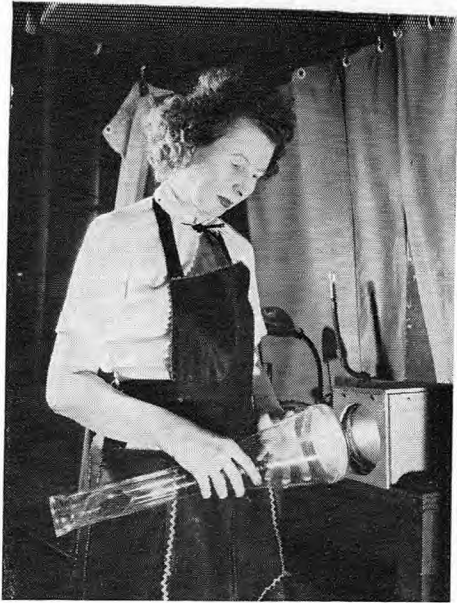
After coating, the screen of the tube bulb is excited by ultra-violet light to inspect for flaws in the screen or screen coating
