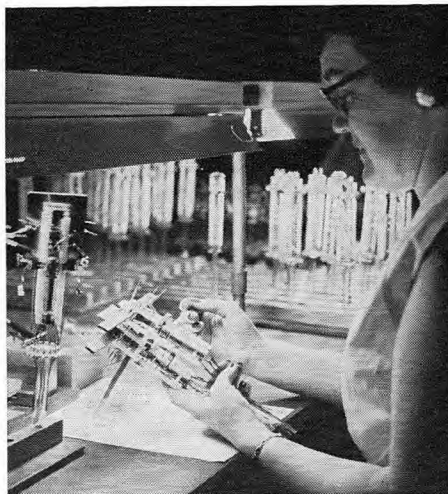
Final inspection of a Type 55P-A dual-gun with "go-no go" gages. The inspector checks for spacings, alignment of electrodes, and for specification qualifications in general
