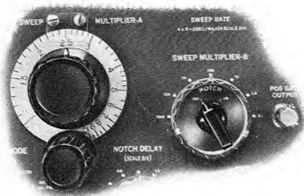
Figure 6. By multiplying two readings, from vernier dial MULTIPLIER A, and the stepped switch MULTIPLIER B, the time between major scale divisions is precisely determined. To measure the duration of a pulse, merely adjust the vernier until the pulse occupies a major scale division, then read the pulse width as the product of A \times B . The multiplication is easy since MULTIPLIER B reads in decade steps
