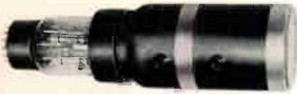
Figure 1. Type K1098P-, containing four wholly independent electron-gun and deflection-electrode structures.
